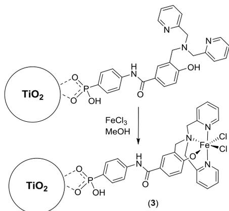
**Fig. 3.** Assembly of iron catalyst (**3**) on TiO<sub>2</sub>.
