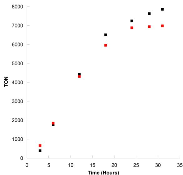
**Fig. 5.** Hydrogen generation from **3**-TiO<sub>2</sub> (black) and **3**-SrTiO<sub>3</sub> (red) with 2 mM fluorescein and 5% TEA in 1:1 ethanol:water.
