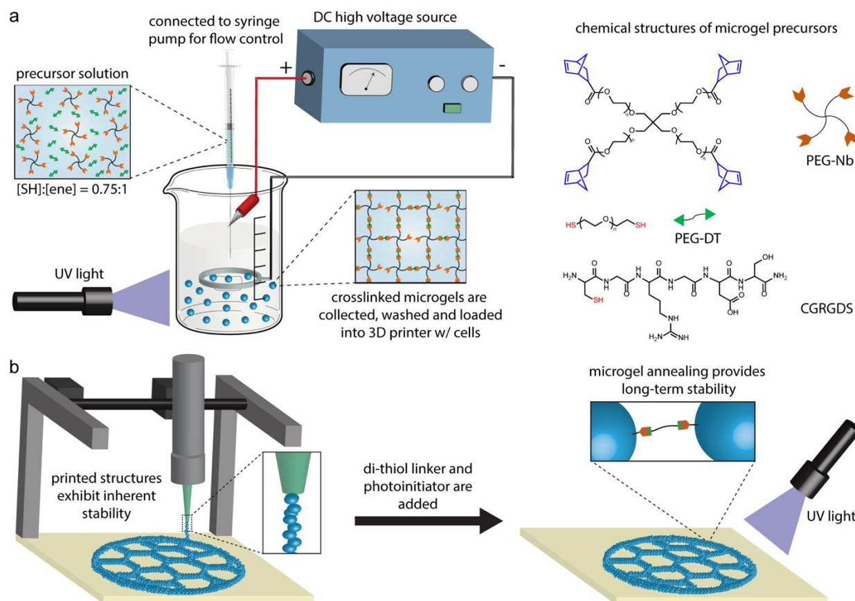
**Figure 1.** Overview of clickable PEG microgel bioink production and use in 3D printing. a) Chemical structures and schematic of the submerged electro spraying setup for synthesizing PEG microgels via thiol-ene click chemistry. b) Schematic of PEG microgel 3D printing procedure. Printed structures exhibit inherent stability due to the cohesive forces between PEG microgels. Long-term stability is achieved by annealing the microgels with a second thiol-ene reaction that crosslinks the microgels.
