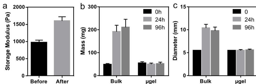
**Figure 5.** Crosslinked constructs from microgel bioinks exhibit enhanced mechanical properties and non-swelling properties. a) Storage modulus of printed microgel disks before and after photopolymerization. The swelling properties were compared between bulk hydrogel and microgel printed disks as measured in b) mass and c) diameter.
