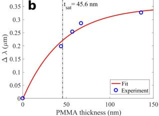
**Fig. 4** Measurements of the penetration depth  $t_{\rm sat}$  of the metasurface evanescent field using variable-thickness PMMA coverage. The wavelength shift  $\Delta\lambda$  of the reflectivity maximum for (a) Pixel 1, and (b) Pixel 2 depends on the PMMA thicknesses t. At  $t=t_{\rm sat}$  the shift reaches 63% of its asymptotic value.
