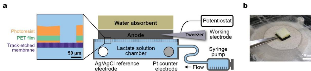
**Fig. 2** (a) Schematic diagram of the perspiration device and the experimental setup for measuring the anode with a continuous supply of lactate solution. (b) Photograph of the LOx anode placed on the surface of the perspiration device.
