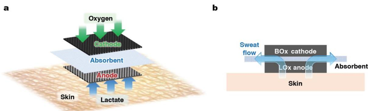
**Fig. 1** Schematic structure of the mesh-type enzymatic biofuel cell for lactate sensing in perspiration. (a) Perspective view. (b) Cross sectional view.
