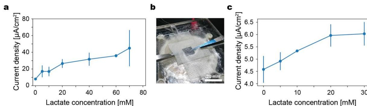
**Fig. 5** (a) Amperometric response of the LOx anode to solution with various concentrations of lactate tested on the perspiration device. (b) Photograph of the self-powered EBFC sensor assembled on an artificial perspiration device. Error bars are standard deviation of 2 or 3 LOx anode samples. (c) Generated electric current of the self-powered EBFC sensor for solution with various concentrations of lactate tested on the perspiration device. Error bars are standard deviation of 2 EBFC samples.
