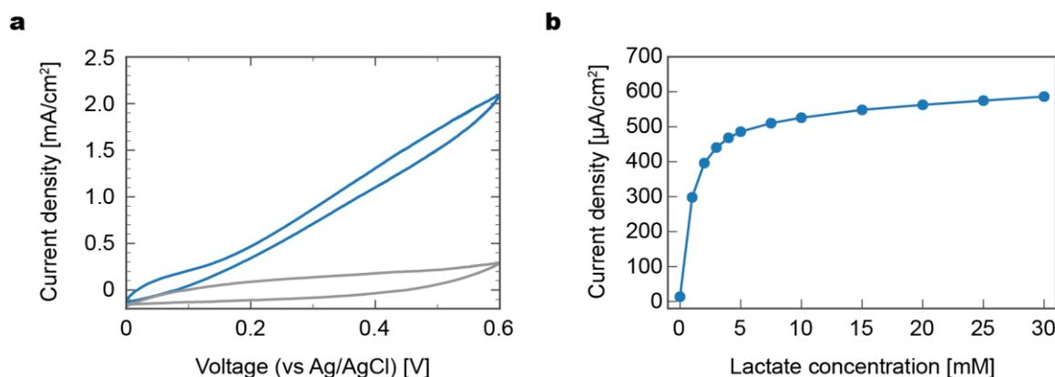
**Fig. 3** Characteristics of a pristine lactate anode without polyurethane coating. (a) Cyclic voltammetry of an anode with 20 mM lactate (blue) and without lactate (gray) in 100 mM phosphate buffer solution (pH 7.0). (b) Current versus lactate concentration in 100 mM phosphate buffer solution (pH 7.0).
