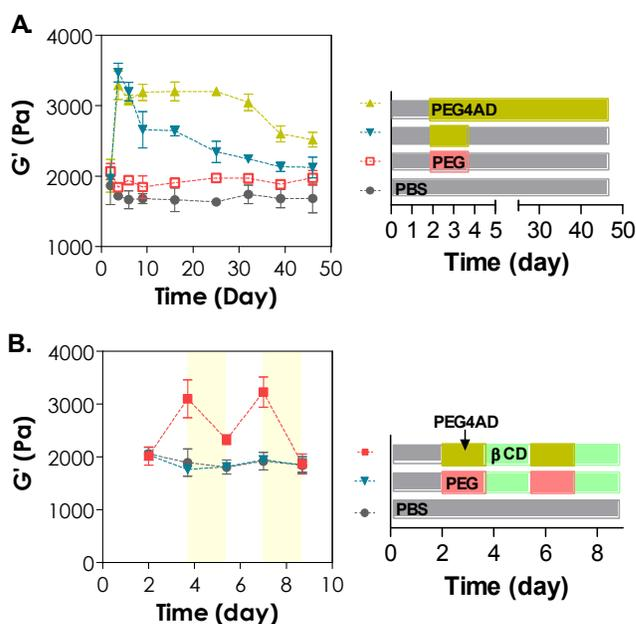
**Fig. 3** (A) Effect of gel treatment conditions on the elastic modulus of thiol-allylether hydrogel. Right panel: timeline for the treatments of hydrogels. (B) Reversibly tuning the elastic moduli of thiol-allylether hydrogel. 5 wt% of PEG4AD (10 kDa) and 5 wt% of 4-arm PEG (10 kDa), respectively. Right panel: timeline for the treatments of hydrogels (2.5 wt% TPVA, 0.8 mM PEG4AE and 27.6 mM  $\beta$ CDAE, Mean  $\pm$  SD, N = 3, \* indicates  $p < 0.05$ ).
