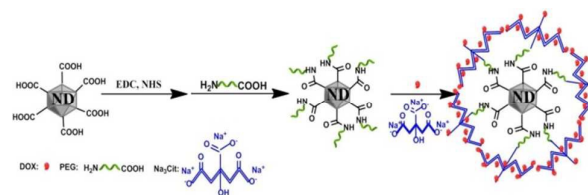
Scheme 2 The preparation of NPDC nanoparticles
