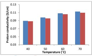
Figure 11. Nafion 117, 0.5% loading. Proton conductivity of MEAs determined using impedance spectroscopy at OCV with a 4M methanol feed at a range of operating temperatures and mordenite loading in the composite layer.
