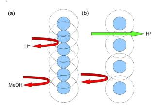
**Figure 14 (a)** A coherent mordenite layer prevents the passage of protons whereas; **(b)** a dispersed composite structure which features an ideal dispersion of mordenite in Nafion could allow the transport of protons through the Nafion and a sphere of organic influence formed by preferentially absorbed water and/or the repulsion of methanol preventing the flow of methanol into the bulk membrane.
