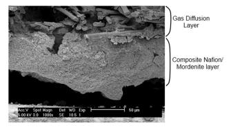
**Figure 7.** Cross sectional view of a composite layer (0.5% functionalised H-mordenite) on the surface of a gas diffusion layer obtained using scanning electron microscopy of a cryogenically fractured sample.
