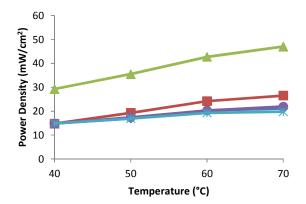
Figure 4. DMFC peak power densities with a 4 M methanol feed. ◆ Nafion 117, 0.25% loading, ▲ 0.5% loading, ● 0.75% loading, ■ 1% loading using a standard MEA and MEAs featuring a mordenite composite layer with a range of mordenite loadings (from 0.25 % to 1.0 %).
