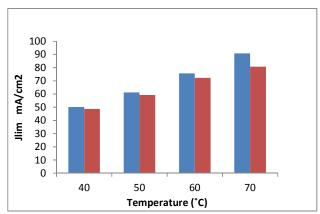
Figure 12. Nafion 117, 0.5% loading. Crossover current density as a function of temperature for a DMFC using a standard Nafion 117 MEA and an MEA containing a 0.5% mordenite with a composite layer.
