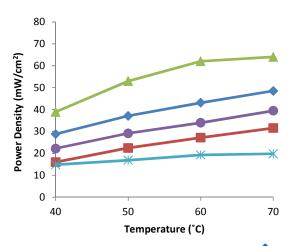
Figure 3. DMFC peak power densities with a 2 M methanol feed. ◆ Nafion 117,
