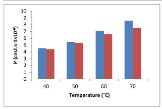
Figure 13. Nafion 117, 0.5% loading. Methanol permeability as a function of temperature for a DMFC using a standard Nafion 117 MEA and an MEA containing a 0.5% mordenite with a composite layer.
