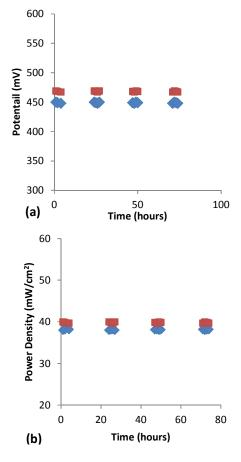
**Figure 6.** DMFC, ◆ Nafion 117, ■ 0.5% loading (a) potential and (b) power density variation during 100 hour operation using a single cell DMFC operating at 70°C, 1 M methanol feed, and at a current of 80 mA cm<sup>-2</sup>.
