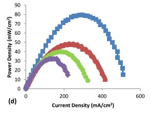
Figure 1. Experimental results showing DMFC performance for a standard Nafion 117 MEA.
