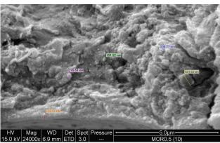
**Figure 8.** Cross sectional view of a 13.2% mordenite/Nafion composite layer sprayed onto glass, obtained using scanning electron microscopy of a cryogenically fractured sample. (NB This composition would give 0.5% functionalised H-mordenite if part of a complete MEA)
