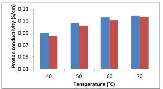
Figure 10. Nafion 117, 10.0.5% loading. Proton conductivity of MEAs determined using impedance spectroscopy at OCV with a 2M methanol feed at a range of operating temperatures and mordenite loading in the barrier layer.
