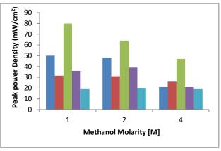
Figure 5. Nafion 117, 0.25% loading, 0.5% loading, 0.7% loading. and 1% loading. Peak power densities for DMFCs using a range of different MEAs, operating at 70°C with 1M, 2M and 4M methanol feed.
