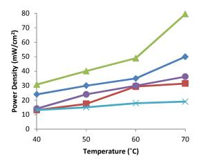
Figure 2. Experimental results showing peak power densities for a DMFC with a 1 M methanol feed. ◆ Nafion 117, ■ 0.25% loading, ▲ 0.5% loading, ● 0.75% loading, ● 1% loading, using a standard MEA and MEAs featuring a mordenite composite layer with a range of mordenite loadings (0.25 % to 1.0 %).
