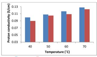
Figure 9. Nafion 117, 0.5% loading. Proton conductivity of MEAs determined using impedance spectroscopy at OCV with a 1M methanol feed at a range of operating temperatures and mordenite loading in the barrier layer.
