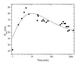
**Fig. 9** Dynamic light scattering data where the aggregate size evolution is monitored with time for SP+ particles and the waxy starch, at a particle to starch ratio corresponding to approximately 1:1 in charge ratio. The line is a guide for the eye.
