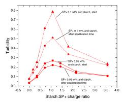
**Fig. 4** Turbidity curves for two different SP+ particle concentrations, 0.05 wt% and 0.1 wt% when combined with the regular starch. The highest SP+ particle concentration gives the highest turbidity increase. The initial turbidity increase is more pronounced for the highest particle concentration.
