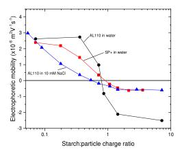
**Fig. 1** Plot of electrophoretic mobility versus starch:particle charge ratio for amidine particles and SP+ particles. The regular starch was used in this part of the study.
