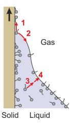
**Figure 6**: Schematic of processes at the receding contact line. Details are explained in the main text.
