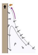
**Figure 1**: Schematic microscopic picture of the region around the three-phase contact line of a surface drawn out of a liquid pool. The gray arrow indicates the liquid flow, while the surface is pulled upwards (black arrow) and fresh liquid-air interface is created (orange arrow). This fresh interface has a lower surfactant concentration, leading to a Marangoni tension slowing down the liquid flow (purple arrow).
