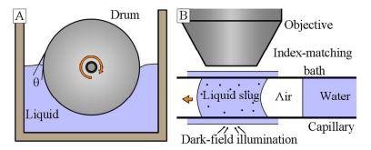
**Figure 2.** A) The rotating cylinder setup in side view to measure the contact angle and track the particle flow inside a dewetting liquid. B) The micro tubing setup for measuring flow profiles close to the three-phase contact line using a liquid slug flowing through a capillary.
