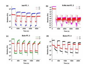
**Fig. 6** Thixotropy tests performed on hydrogels **1** – **4**. After gelation, storage modulus (G') and loss modulus (G'') measurements were performed at a constant frequency (1 Hz) using low strain (0.5%, 600 seconds) followed by high strain (100%, 200 seconds). This protocol was repeated six times. Gels were prepared at 0.6% (w/v) and measurements performed at a constant temperature of 25 °C.
