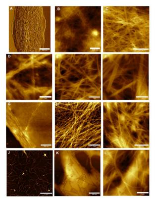
Fig. 7 AFM images of the gel networks of 1 - 4 evolving with concentration. 1 at concentrations of 0.1, 0.5 and 1% (w/v) (a-c), 2 at concentrations of 0.1, 0.5 and 1% (w/v) (d-f), 3 at concentrations of 0.01, 0.02 and 0.1% (w/v) (g-i) and 4 at concentrations of 0.02, 0.1 and 0.2% (w/v) (j-I). All samples were spread coated onto a freshly cleaved mica substrate. Scale bars denote 500 nm (A – C), 1  $\mu$ m (D – F, H, J, L) and 300 nm (G, I, K).
