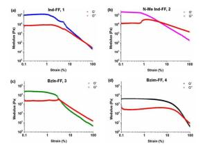
Fig. 4 Strain sweeps performed on hydrogels 1 - 4. Gels were prepared at 0.6% (w/v) and storage (G') and loss modulus (G'') measurements performed at a constant frequency of 1 Hz and temperature of 25 °C.
