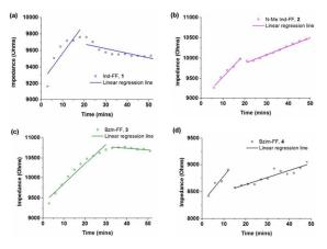
Fig. 3 Time dependent impedance data for 1 - 4. Measurements were performed at 25 °C and impedance data was averaged over 0.1 to 100 kHz, where the impedance is independent of frequency.
