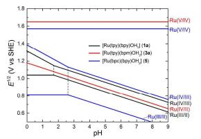
**Figure 3.** Pourbaix diagrams for  $[Ru(tpy)(bpy)OH_2]^{2^+}$  (1a),  $[Ru(tpy)(bpm)OH_2]^{2^+}$  (3a) and  $[Ru(bpc)(bpy)OH_2]^{2^+}$  (5); solid lines indicate trends of redox potentials depending on pH; dotted lines indicate  $pK_a$  of  $[Ru^{III}-OH_2]$  species. The diagram was drawn according to reported experimental data in references. <sup>38,42,43</sup>
