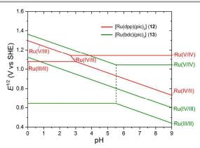
**Figure 5.** Pourbaix diagrams for  $[Ru(dpp)(pic)_2]^{2+}$  (**12**) and  $[Ru(bdc)(pic)_2]$  (**13**); solid lines indicate trends of redox potentials depending on pH; dotted lines indicate  $pK_a$  of  $[Ru^{III}-OH_2]$  species. The diagram was drawn according to reported experimental data in references. <sup>64,65</sup>
