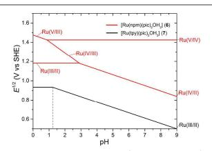
**Figure 4.** Pourbaix diagrams for  $[Ru(npm)(pic)_2OH_2]^{2+}$  (6) and  $[Ru(tpy)(pic)_2OH_2]^{2+}$  (7); solid lines indicate trends of redox potentials depending on pH; dotted lines indicate  $pK_a$  of  $[Ru^{III}-OH_2]$  species. The diagram was drawn according to reported experimental data in the reference. <sup>55,57</sup>
