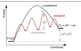
**Figure 1**. Schematic energy profiles for the uncatalyzed and catalyzed water to dioxygen reaction. The highest energy barrier ( $\Delta G^{\dagger}$ ) in the catalyzed path is marked. The transition state is denoted as TS.
