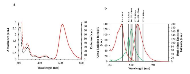
**Figure 2**: (a) Absorbance and emission properties of Ru-NLS in MeCN (—) and water (—) displaying the 'light switch' effect. (b) Spectral rationale of confocal and STED setup. Ruthenium excitation and emission (—), and AlexaFluor Fluor 532 excitation and emission spectra (—), in aerated PBS solution.
