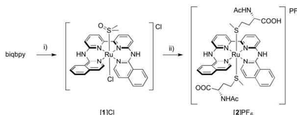
Scheme 1. Synthesis of [1]Cl and [2]PF<sub>6</sub>. Conditions: i) 1.1 eq. [Ru(DMSO)<sub>2</sub>Cl<sub>2</sub>], 80 °C, in EtOH under argon, 16 h, yield 43%; ii) 20 eq. HAmet, 80 °C, in water under argon, 16 h, yield, 43 %.
