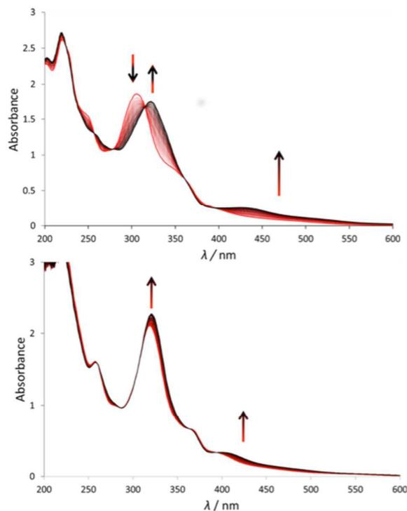
Figure 2. Evolution of the electronic absorption spectra of a solution of [1]Cl (a) and [2](PF<sub>6</sub>) (b) in demi-water upon green light irradiation under argon ( $\lambda = 530$  nm,  $\Delta\lambda_{1/2} = 25$  nm, 3.02 mW,  $2.1 \times 10^{-8}$  Einstein.s<sup>-1</sup>). Time: 0 min (red curve) to 120 min (black curve, a) or 160 min (black curve, b). Conditions [Ru]<sub>0</sub> =  $7.5 \times 10^{-5}$  (a),  $7.8 \times 10^{-5}$  (b), irradiated volume was 3.0 mL at 298 K.
