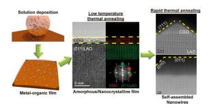
A novel approach to perform an independent study of the nucleation and coarsening of  $Ce_{0.9}Gd_{0.1}O_{2\text{-y}} \text{ nanowires is presented.}$
