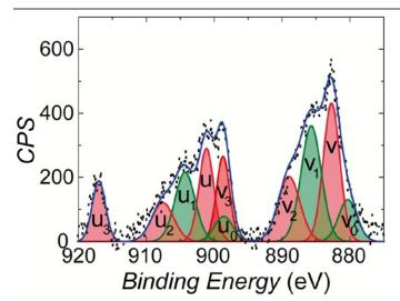
Figure 4. XPS Ce 3d core level spectrum of (011)CGO nanowires grown on (011)LAO substrates by RTA at 1000  $^{\circ}$ C, 20  $^{\circ}$ C s<sup>-1</sup> for 5 min in O<sub>2</sub> atmosphere. The fitted components in green and red correspond to Ce<sup>3+</sup> and Ce<sup>4+</sup> ions, respectively.
