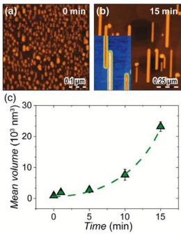
**Figure 8.** AFM images showing the evolution of nanowires grown in O<sub>2</sub> at 1000 °C: (a) 0 min, and (b) 15 min of annealing. Inset: two close NWs illustrating the presence of elastic repulsive interactions. (c) Evolution of the mean volume of a single NW with time from 0 to 15 min.
