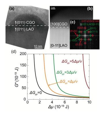
**Figure 6.** (a) HRTEM image of a short length (011)CGO island on (011)LAO. (b) HAADF-STEM characterization, and (c) power spectrum of an equivalent island viewed from the [100]CGO//[0-11]LAO zone axis. The sample was grown at 1100  $^{9}$ C, 20  $^{9}$ C s<sup>-1</sup> for 5 min in O<sub>2</sub>. (d) Dependence of the nucleation barrier ( $G^*$ ) with the supersaturation ( $\Delta\mu$ ) for different strain contributions ( $\Delta G_{ST}$ ).
