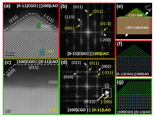
Figure 3. (a) Cross-sectional HAADF STEM image of a (011)CGO nanowire (front view) viewed from the [0-11]CGO//[100]LAO zone axis. (b) Power spectrum obtained from the HAADF STEM image in (a). (c) Cross-sectional HAADF STEM image of a (011)CGO nanowire (lateral view, longitudinal) viewed from the [100]CGO//[0-11]LAO zone axis. (d) Power spectrum obtained from the HAADF STEM image in (c). (e) 3D atomic model of a CGO NW on a LAO substrate, and corresponding (f) front and (g) lateral views.
