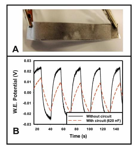
Figure 11 A photograph of a solid state P-SC, using an H2SO4-PVA electrolyte, A), and the characteristic charge performance of the device with a 5  $\mu$ A charging current, B).
