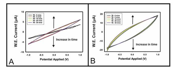
Figure 4 Voltammograms of the 7B pencil drawn electrodes, in  $0.1 \text{ M H}_2\text{SO}_4$  aqueous solution, over the range -1.0 to 1.0 V, both single sided, A), and double sided, B) interdigitated pencil drawn electrodes.
