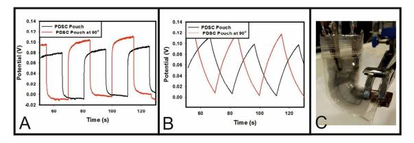
Figure 10 Charge/discharge characteristics of the P-SC; A) Without the circuit, B) with the circuit of capacitance 620  $\mu$ F, C) a photograph of the bent P-SC held in position by a clamp.
