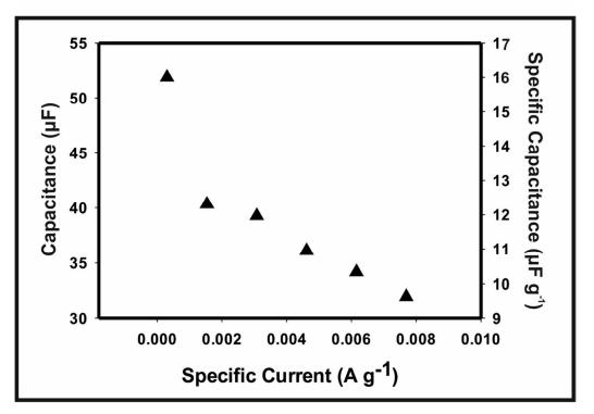
Figure 7 Plot for the effect on the capacitance of the double-sided 8B pencil drawn electrode in 0.1M H<sub>2</sub>SO<sub>4</sub>.
