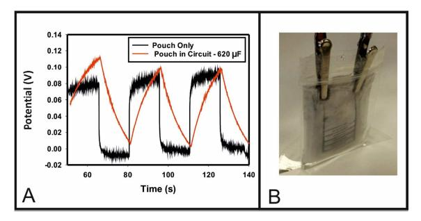
**Figure 8** A) The charge-discharge characteristics of the pouch capacitor, both without the parallel circuit, and with a circuit capacitance of 620  $\mu$ F. B) A photograph of the pouch arrangement, the pouch consists of 5 double sided 8B pencil drawn electrodes in parallel, with paper spacers between each, the pouch is filled with 3 ml of 0.1 M of H<sub>2</sub>SO<sub>4</sub>.
