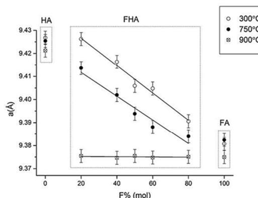
**Fig. 2.**  $a$  axis unit cell parameter plotted against F%,  $a$  axis reducing with increasing F% but becoming independent of F% in  $900^\circ\text{C}$  series. The lines represent linear fits of the data. The equations are given in supporting material table S1.
