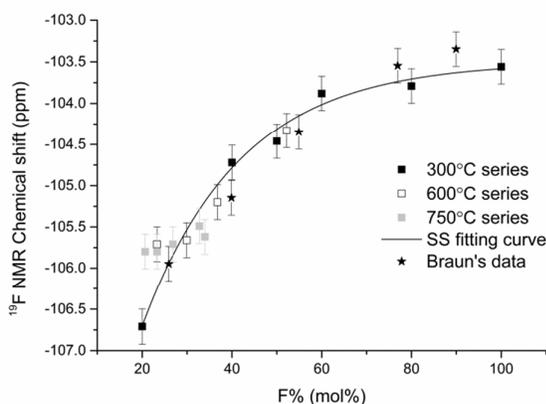
**Fig. 8.** <sup>19</sup>F NMR Chemical shifts plotted against F% and the fitting curve of the 300°C series (SS fitting curve): Four sets of data are presented: three of them from the project (300, 600 and 750°C series), and the fourth set of data from Braun's work is also plotted for comparison
