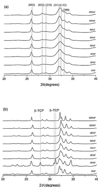
**Fig. 1.** XRD patterns of (a) 300 (b) 750 and (c)  $900^\circ\text{C}$  samples. The  $h, k, l$  indices shown in (a) are also true for the diffraction lines in (b) and (c).
