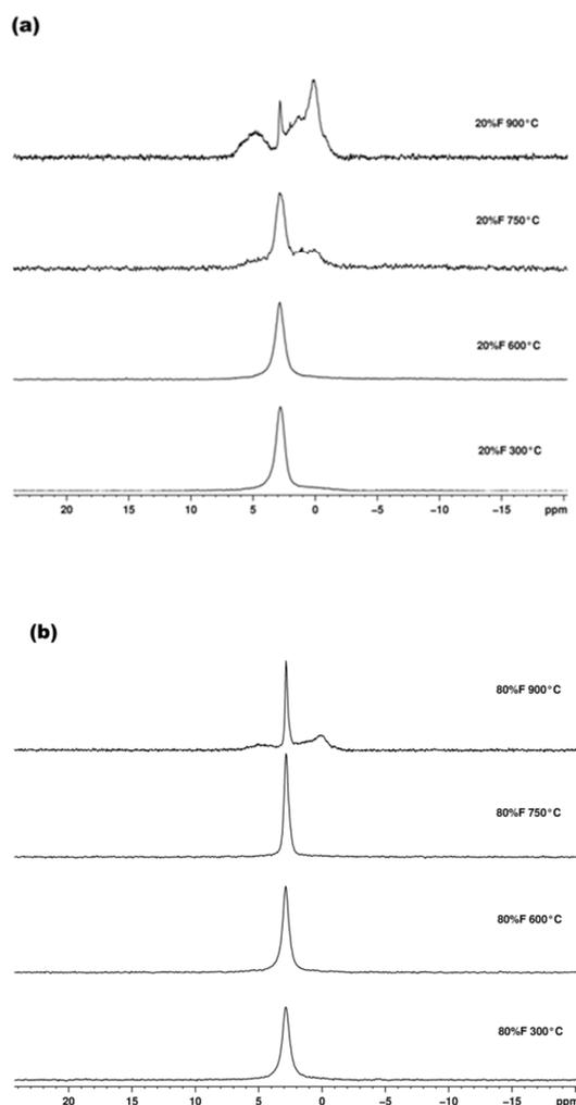
**Fig. 10.**  $^{31}\text{P}$  MAS-NMR spectra of 20 and 80%F at different heat treatment temperature (a) 20%F heat treated from 300 to 900°C,  $\beta$ -TCP are observed from 750°C (b) 80%F heat treated from 300 to 900°C,  $\beta$ -TCP are observed at 900°C
