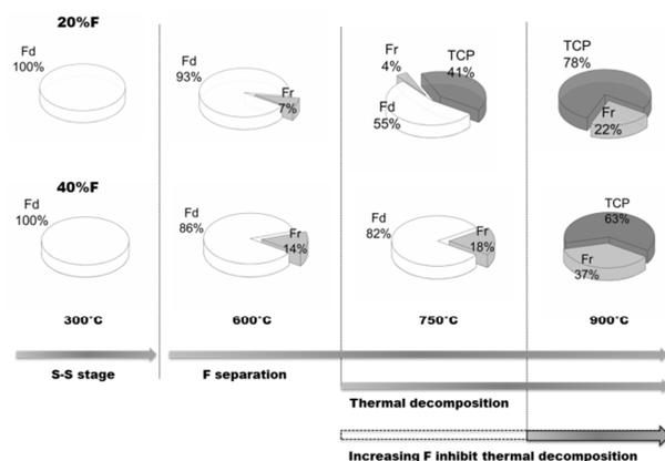
**Fig. 7.** Compositions changing of 20 and 40%F samples with increasing heat-treatment temperature from 300 to 900°C. The β-TCP percentage comes from the XRD refinement data (Fig. 3) and the Fr and Fd percentage were calculated by <sup>19</sup>F NMR deconvolution results (table 2).
