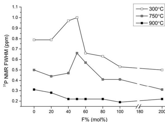
**Fig. 5.** The fwhm of  $^{31}\text{P}$  MAS-NMR signal of FHA heat treated at 300, 750 and 900°C. The linewidth narrows with increasing heat treatment temperature, at 900°C, the fwhm stabilizes at 0.22ppm.
