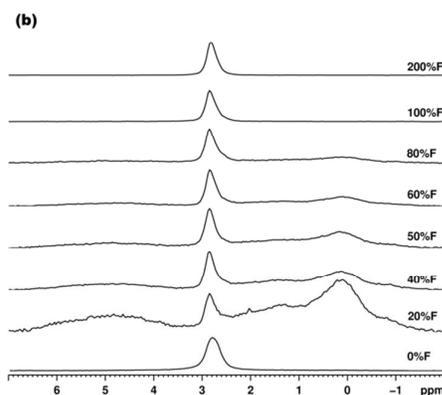
**Fig. 4.**  $^{31}\text{P}$  MAS-NMR spectra of FHA (a) Heat treated at 300°C, main resonance centred at 2.8ppm corresponding to the  $\text{PO}_4^{3-}$  in apatite structure (b) Heat treated at 900°C, the main resonance at 2.8ppm, another additional broad resonance at 0.1-5.0 ppm corresponding to  $\text{PO}_4^{3-}$  in  $\beta$ -TCP are observed in 20 to 80%F
