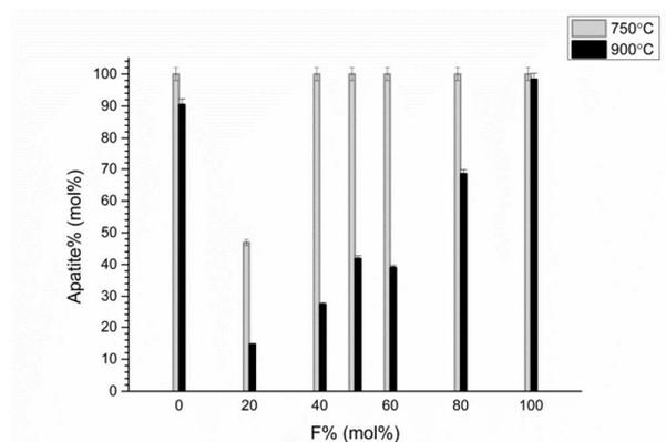
**Fig. 3.** Comparison of the amount of apatite phase between 750 (grey bar) and 900°C (black bar), most of XRD patterns at 750°C contain single apatite phase; most of apatite phases at 900°C show decomposition (20 to 80%F).
