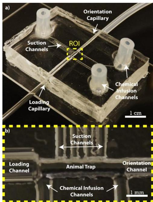
Figure 1. (a) Hybrid microfluidic chip used for 3<sup>rd</sup> instar *Drosophila* larva orientation, immobilization, chemical exposure, and monitoring of cardiac activities. Loading and orientation glass capillaries were installed in the corresponding guide channels shown in (b) and rotated manually for larva orientation. Region of Interest (ROI) in (a) is magnified in (b).
