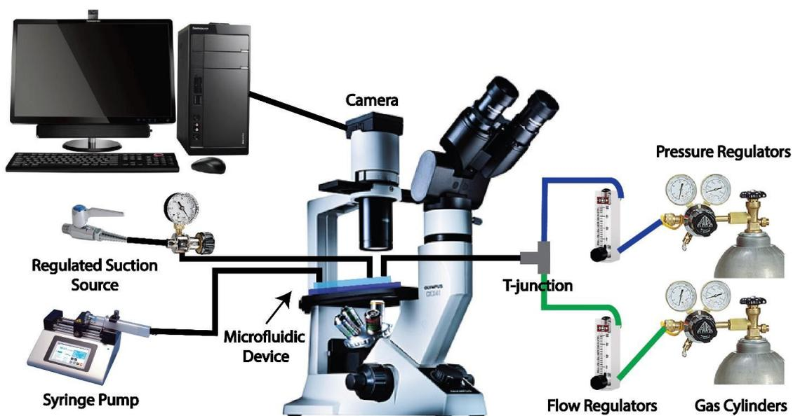
Figure 2. Experimental set-up consisting of three main units, i.e., animal handling, chemical delivery, and monitoring and imaging units. Animal handling unit included two syringes connected to loading and orientation glass capillaries on the microfluidic device and a regulated suction source. Chemical delivery unit consisted of a syringe pump, gas cylinders, flow and pressure regulators, and a T-junction. Monitoring and imaging unit consisted of a microscope, a camera and a computer.
