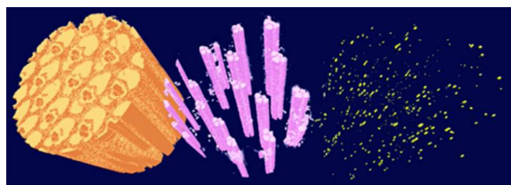
Fig. 8 One frame picture of the on-line video showing different physical parts of the biocomposite engineered material: sclerenchyma and parenchyma tissues (orange); metaxylem, phloem and protoxylem vessels (purple) and silver aggregates (yellow).
