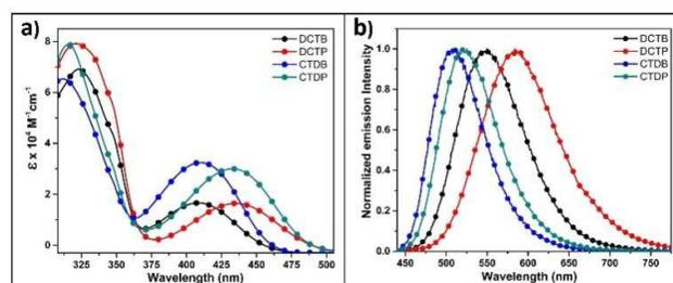
Fig. 4 a) Absorption and b) emission spectra of dyes ( $1 \times 10^{-5}$  M) recorded in toluene at ambient temperature.
