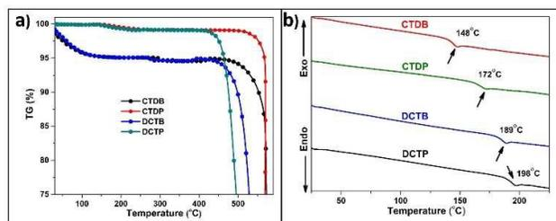
**Fig. 7.** Thermograms (a) and DSC traces (b) of the dyes measured at a heating rate of 10 °C/min under N<sub>2</sub> atmosphere.
