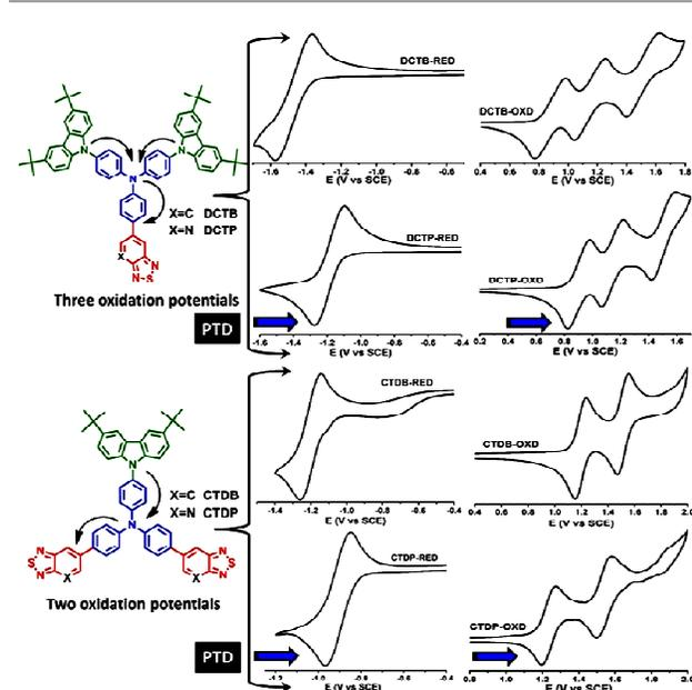
**Fig. 6.** Cyclic voltammograms of the dyes recorded in dichloromethane.
