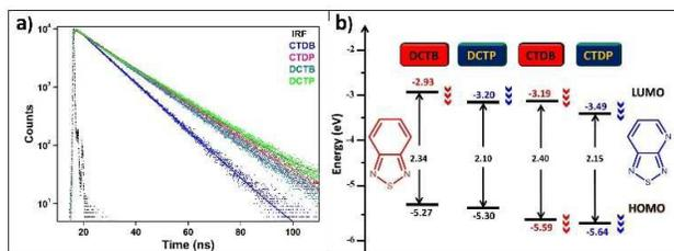
**Fig. 5.** a) Time-resolved fluorescence decay curves of the dyes in toluene ( $\lambda_{\text{ex}} = 405 \text{ nm}$ ,  $\lambda_{\text{em}} = 530 \text{ nm}$ ); b) Schematic diagram represents the modulation of energy levels estimated from electrochemical data.
