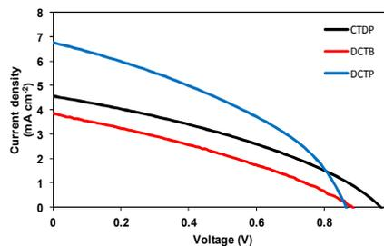
**Fig. 8.** Characteristic current density versus voltage ( $J$ - $V$ ) curves for the best BHJ devices based on CTDP (black), DCTB (red) and DCTP (blue) in blends with PC<sub>61</sub>BM under simulated sunlight (100 mWcm<sup>-2</sup>, AM 1.5G). The device structure is: ITO/PEDOT:PSS (38 nm)/active layer/Ca (20 nm)/Al (100 nm).
