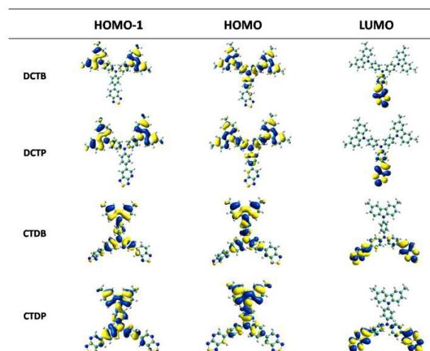
Fig. 3. Computed isodensity (0.02) surfaces of the HOMO-1, HOMO and LUMO of the target molecules.
