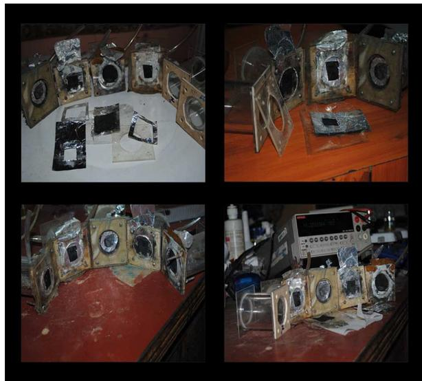
**Fig 11: Membrane electrode assemblies (MEA) in single chambered MFCs**
