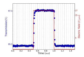
**Figure.5** Transmission versus time of a CdSe/CdS NR suspension in dodecane when a pulse with amplitude of 17 V/um is applied.
