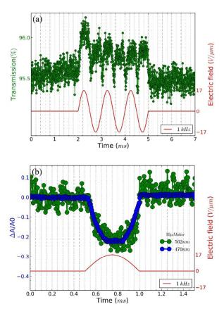
**Figure 6.** (a) Transmission measurement (green dots) of a NR suspension for green (~560 nm) light in the presence of an AC electric field with frequency 1 kHz and amplitude 17 V/ $\mu$ m (red) (b) Relative change of the measured absorbance of the 10  $\mu$ Molar NR dispersion for blue light (blue dots) and green light (green dots) in the presence of an AC electric field with frequency 1 kHz and amplitude 17 V/ $\mu$ m (red).
