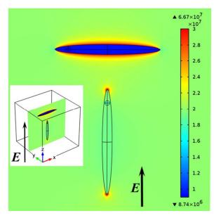
**Figure 7.** Simulation of the field distribution (V/m) inside a dot in rod using the bulk dielectric function for incident light parallel and perpendicular to the c-axis of the rod at 560 nm. The minimum and maximum values of the field are indicated next to the triangles. (Inset: 3D structure shows the position of the NRs in the medium).
