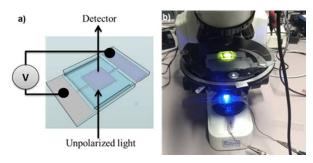
**Figure 2.** a) Schematic view of the cell used to align dispersed nanorods by means of electric fields and (b) image of the microscope transmission setup.
