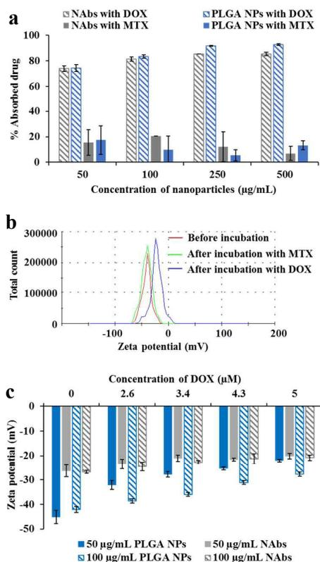
**Fig. 3** Study of chemotherapeutics absorption into the NAbs. (a) Spectrophotometric determination of DOX and MTX absorption into the NAbs and PLGA NPs. (b) Variation in surface charge before and after drug absorption. (c) Changes in the surface charge of NAbs when treated with different concentration of DOX. Value represents mean  $\pm$  s.d.,  $n = 3$ .
