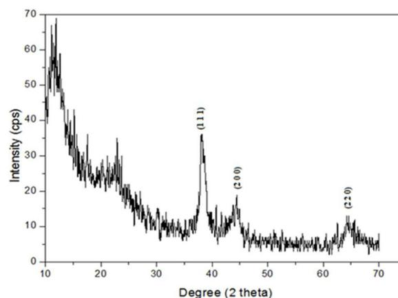
Fig. 5 XRD pattern of DS-Q-GNPs
