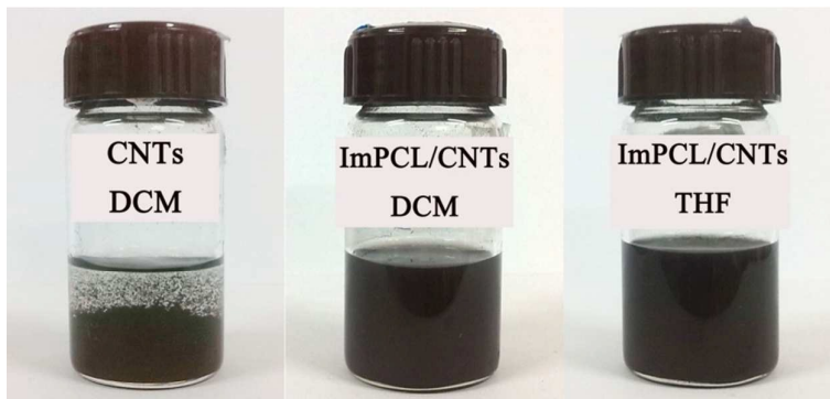
Figure 2. CNTs dispersion test with and without ImPCL in organic solvent
