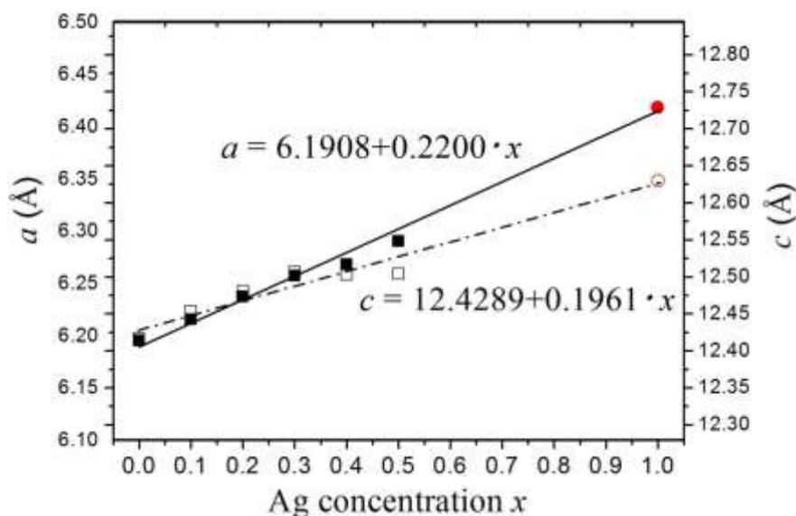
Fig. 3. Variation of lattice parameters  $a$  and  $c$  vs Ag content in the  $\text{Cu}_{1-x}\delta\text{Ag}_x\text{InTe}_2$  ( $x = 0 - 0.5$ ) solid solution.
