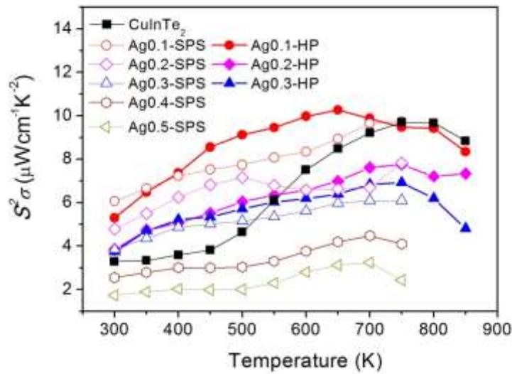
Fig. 6. Power factor as a function of temperature for  $\text{Cu}_{1-x}\text{Ag}_x\text{InTe}_2$  ( $x = 0 - 0.5$ ).
