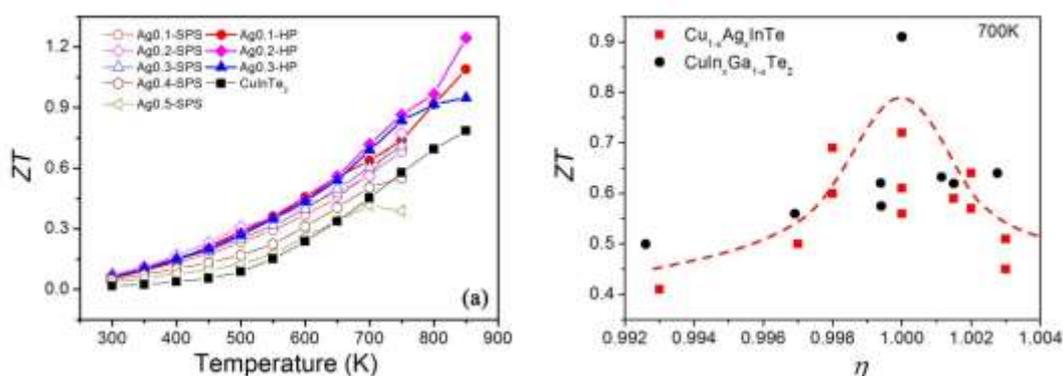
Fig. 12. (a) Dimensional thermoelectric figure of merit as a function of temperature for  $\text{Cu}_{1-x-\delta}\text{Ag}_x\text{InTe}_2$  ( $x = 0 - 0.5$ ); (b)  $ZT$  value as a function of distortion parameter  $\eta$  at 700 K for  $\text{Cu}_{1-x-\delta}\text{Ag}_x\text{InTe}_2$ ,  $\text{CuInTe}_2$ <sup>14, 16</sup>, and  $\text{Cu}(\text{In}_x\text{Ga}_{1-x})\text{Te}_2$ <sup>15, 18, 59</sup>.
