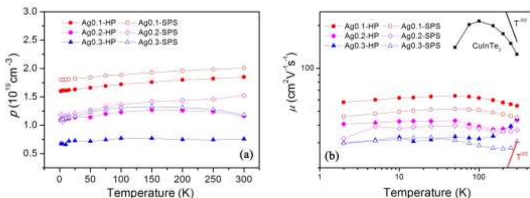
Fig. 7. Temperature dependence of hole concentration  $p(T)$  (a) and hole mobility  $\log\mu$  ( $\log T$ ) (b) for  $\text{Cu}_{1-x}\delta\text{Ag}_x\text{InTe}_2$  ( $x = 0.1 - 0.3$ ) samples.
