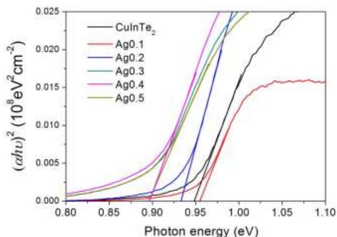
Fig. 4. Photon energy dependence of  $(\alpha h\nu)^2$  for  $\text{Cu}_{1-x}\text{Ag}_x\text{InTe}_2$  ( $x = 0 - 0.5$ ) at room temperature. Extrapolation of the linear part of the dependence to  $(\alpha h\nu)^2 = 0$  yields the estimated band gap  $E_g$ .
