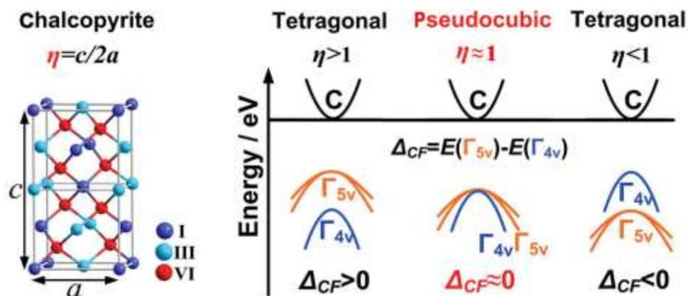
Fig. 1. Crystal structure and electronic bands in ternary chalcopyrites. The pseudocubic structure shows  $\eta \approx 1$ , and the split bands  $\Gamma_{4v}$  and  $\Gamma_{5v}$  nearly degenerate at the top of valence band.
