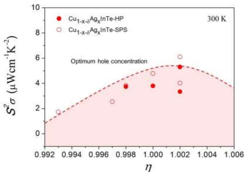
Fig. 9. Power factors as a function of distortion parameter  $\eta$  for  $\text{Cu}_{1-x-\delta}\text{Ag}_x\text{InTe}_2$  ( $x = 0 - 0.5$ ) materials at 300 K. The dashed line is a guide to the eyes, which represents the materials with optimum hole concentrations at various  $\eta$  values.
