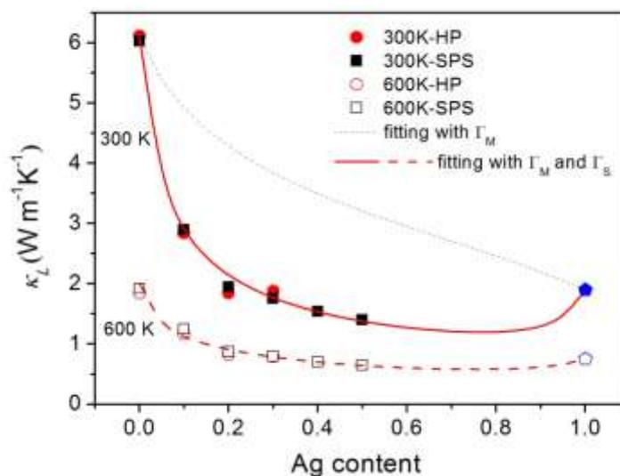
Fig. 11. Lattice thermal conductivity as a function of Ag content in  $\text{Cu}_{1-x}\text{Ag}_x\text{InTe}_2$  ( $x = 0 - 0.5$ ) at 300 K and 600 K<sup>19</sup>. The black dashed line shows the calculated  $\kappa_L$  only based on the mass fluctuation between Cu and Ag at 300 K, and the red lines represent the calculated  $\kappa_L$  including both mass and strain field fluctuations with  $\varepsilon = 280$  at 300 K and 600 K.
