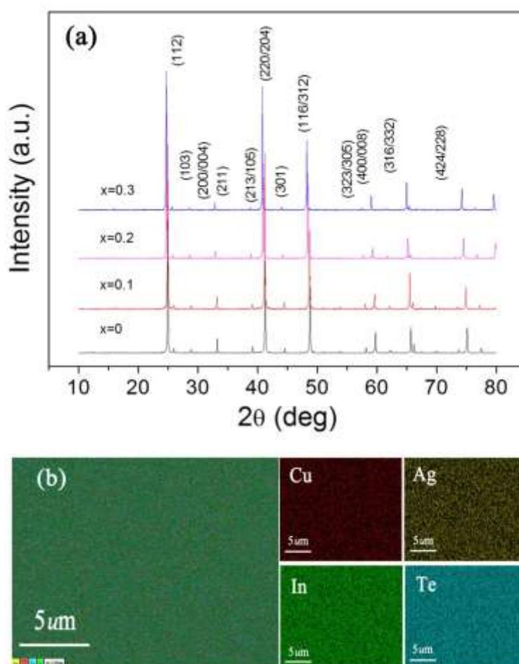
Fig. 2. (a) X-ray powder diffraction patterns of  $\text{Cu}_{1-x}\text{Ag}_x\text{InTe}_2$  solid solution ( $x = 0.1 - 0.3$ ); (b) EPMA-filtered secondary X-ray element maps of HP-  $\text{Cu}_{0.75}\text{Ag}_{0.2}\text{InTe}_2$ .
