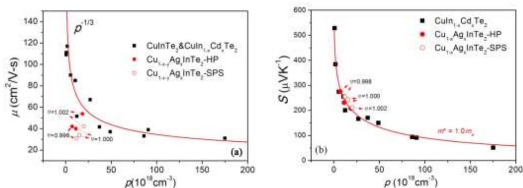
Fig. 8. hole concentration  $p$  dependence of the hole mobility  $\mu$  (a) and Seebeck coefficient  $S$  (b) for  $\text{Cu}_{1-x}\delta\text{Ag}_x\text{InTe}_2$  ( $x = 0 - 0.3$ ) at 300 K. The squares represent experimental data from literature (Refs.14, 18, and 37), and the circles represent our data. The line in (a) gives the  $p^{-1/3}$  relationship, the red lines in (b) were generated using the single parabolic band model by taking  $m^* = 1.0m_e$  respectively.
