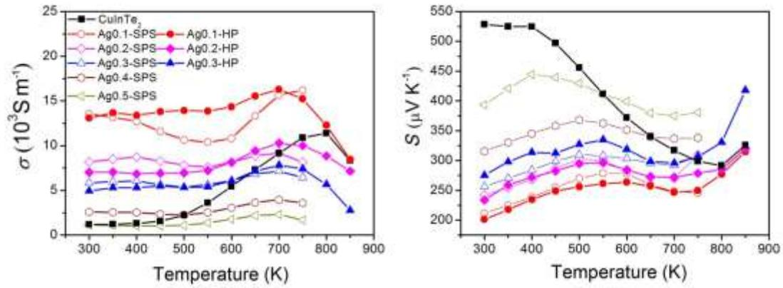
Fig. 5. Temperature dependence of electric transport properties of polycrystalline  $\text{Cu}_{1-x}\text{Ag}_x\text{InTe}_2$  ( $x = 0 - 0.5$ ); (a) electrical resistivity  $\sigma$  and (b) Seebeck coefficient  $S$ .
