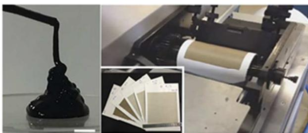
Figure 4 (Left) Viscoelastic property of ( $\sim 40$  mg ml<sup>-1</sup>) GO nematic liquid crystal Scale bar, 1 cm. (Right) Gravure printing machine and (inset) 13  $\times$  14 cm<sup>2</sup> GO membranes with different thicknesses<sup>7</sup> Adapted with permission from Akbari *et al.* (2016); full details are given in the respective publication
