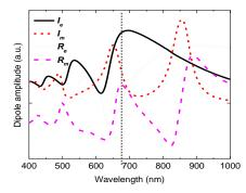
**Figure 4.** Theoretical analysis using the dipole-dipole model. The real and imaginary part of the electric and magnetic dipolar resonances excited in the dimer configuration calculated using the analytical dipole-dipole model.
