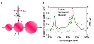
**Figure 9.** (a) Schematic image of the configuration used in calculation. (b) Scattering spectra of the trimer. Scattering cross section to the forward and backward direction and F/B ratio of the trimer using silicon spheres of 165 nm, 225 nm and 310 nm diameter.
