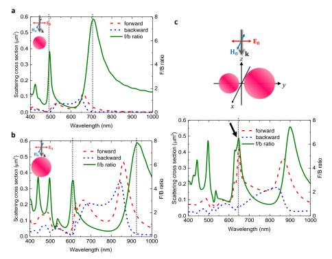
Figure 2. Configuration and results of the FDTD simulation. (a-c) Spectra of scattering cross section to the forward and backward direction and F/B ratio of the 165 nm diameter single sphere (a), the 225 nm diameter single sphere (b) and the dimer of these spheres (c). Insets are configurations used in the calculation.
