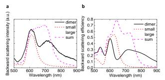
**Figure 8** Comparison of experimental (a) and theoretical (b) scattering spectra to the backward direction of the single disks, the numerical sum of these two disks and the dimer configuration.
