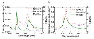
**Figure 6.** Scattering properties shifted to the boundaries of the visible regime. Spectra of scattering cross sections to the forward and backward directions and F/B ratio of the dimer using silicon spheres of 110 nm and 150 nm diameter (a) and the dimer using silicon spheres of 225 nm and 310 nm diameter (b).
