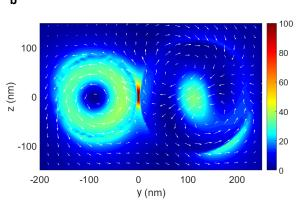
**Figure 3.** (a) Scattering pattern in far field from the single spheres and dimer configuration projected in x-z plane. (b) Electric field intensity and coupling between the resonances. Cross section of electric field intensity inside and near the dimer configuration at 647 nm illumination in the y-z plane. White arrows in the figure show the real part of electric field vectors at each calculation cell.
