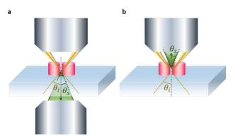
**Figure 1.** Schematic images of the optical measurement setup. Detailed illustration of the darkfield single nanoantenna measurement setups for the forward scattering (a) and backward scattering (b).
