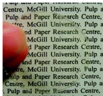
Fig. 17 Transparent film (nanopaper) prepared from drying ENCC. 67 Reprinted with permission from Yang et al., 67 Copyright (2012) American Chemical Society.
