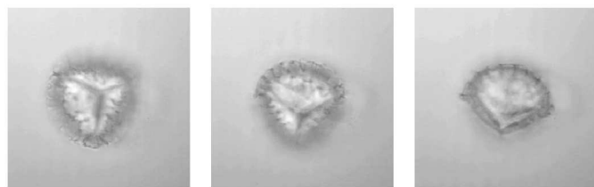
Fig. 3 Lycopodium spore, levitated by acoustic forces and held in place by the optical trap, continuously rotates (image taken from movie, 0.5 s time steps).
