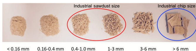
Figure 2: Large particle sizes produced during Wiley milling and sieving.
