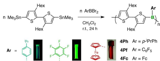
Figure 3. Synthesis and structure of main-chain borane-embedded polythiophenes prepared via tin-boron exchange (Hex = n -hexyl, Fc = ferrocenyl). Adapted with permission from A. Sundararaman, M. Victor, R. Varughese and F. Jäkle, J. Am. Chem. Soc. , 2005, 127 , 13748-13749. Copyright 2005 American Chemical Society.
