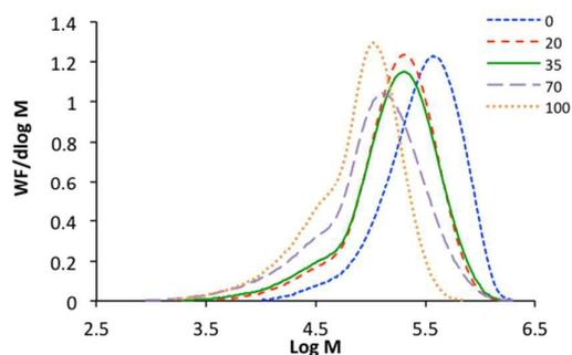
**Figure 4** GPC curves of polyisoprene produced by II/DEAC at different temperatures.
