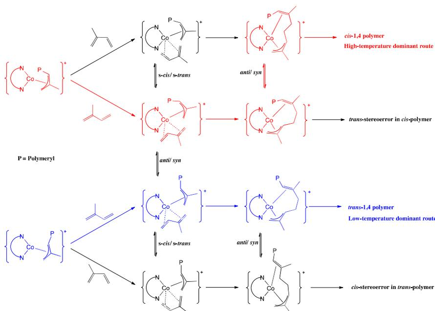
**Scheme 3** Possible Polymerization routes resulting in *cis* or *trans* enchainment of isoprene.
