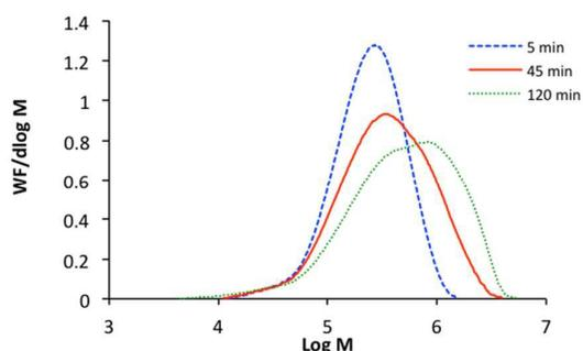
Figure 3 GPC curves of Polyisoprene by **I**/DEAC; for 5, 45 and 120 minutes.
