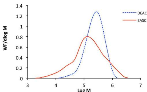
**Figure 5** GPC curves of polyisoprene produced by I/DEAC and I/EASC systems.
