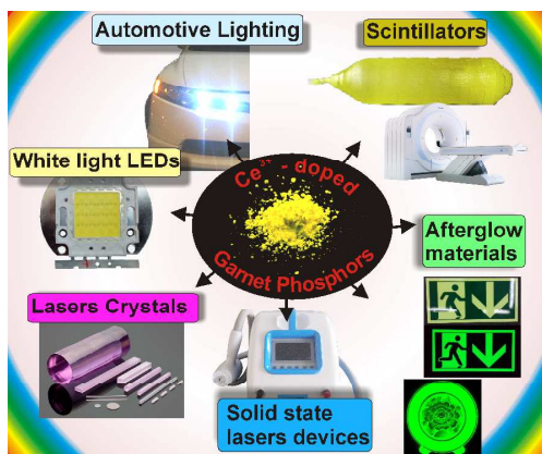
Fig. 2 Some representative application fields of Ce^{3+} -doped garnet phosphors including white light LEDs, scintillators, afterglow materials, laser crystals, and their corresponding applications.
