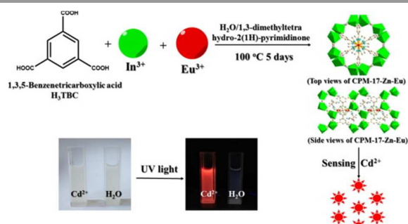
Figure 13. Synthetic procedure of CPM-17-Zn-Eu and its fluorescent enhancement by \text{Cd}^{2+} . 158 Reproduced from Ref. 158 with permission, copyright Elsevier, 2015.
