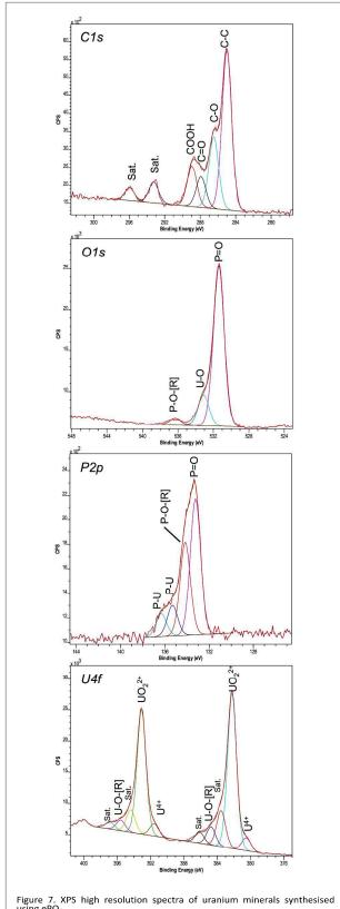
Figure 7. XPS high resolution spectra of uranium minerals synthesised using  $\mbox{ePO}_4$
