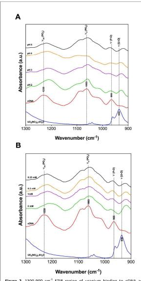
**Figure 2.** 1300-900 cm<sup>-1</sup> FTIR region of uranium binding to eDNA as a function of pH [A] and initial uranium concentration [B].
