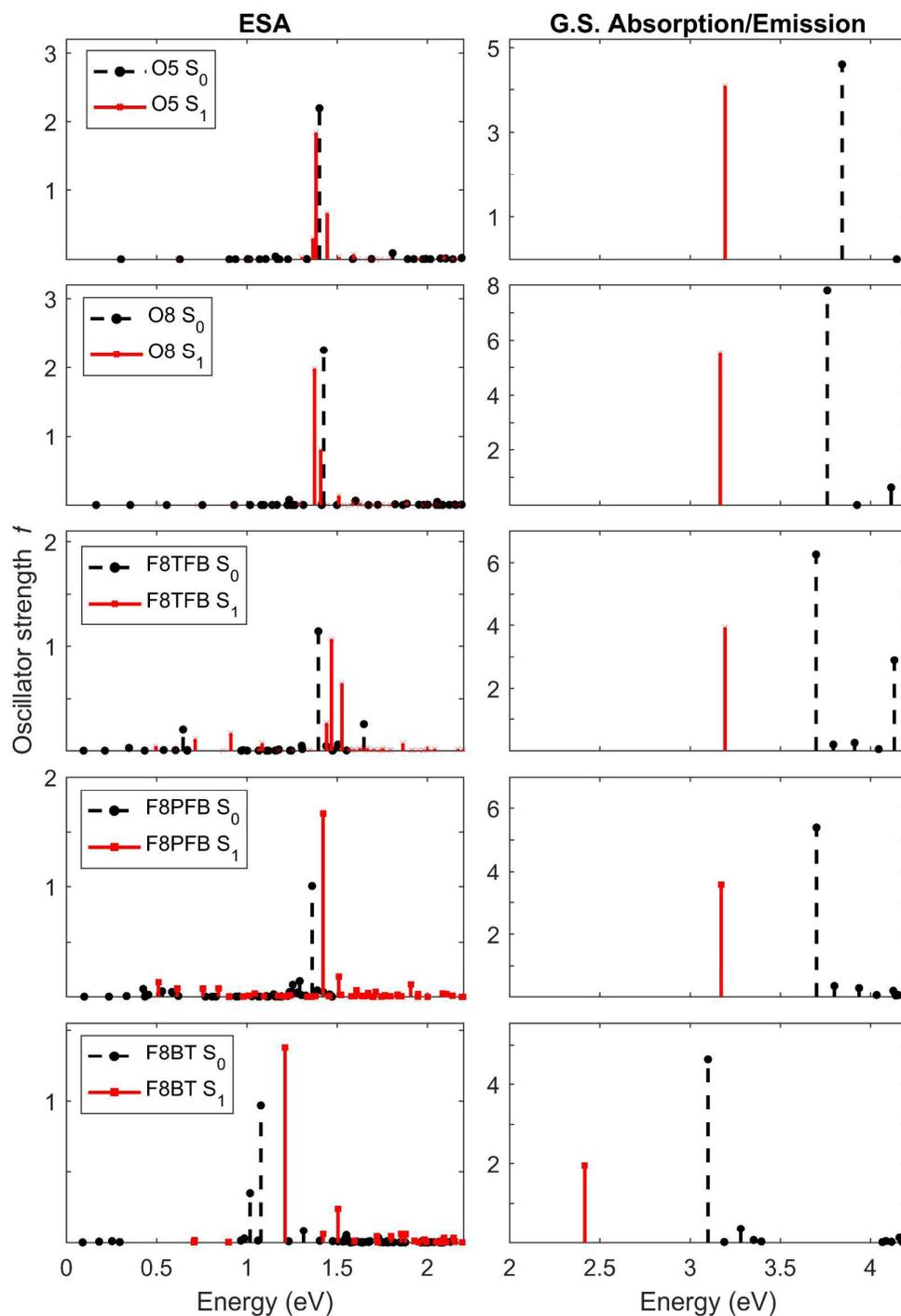
Figure 7: Comparison of the ESA spectra (left panel) calculated for the Franck-Condon state (excited molecule in the ground state geometry), in dashed black lines, and the fully relaxed excited molecule ( $S_1$  geometry), in red solid lines, and the ground-state absorption and emission spectra (right panel), respectively in dashed black lines and red solid lines.
