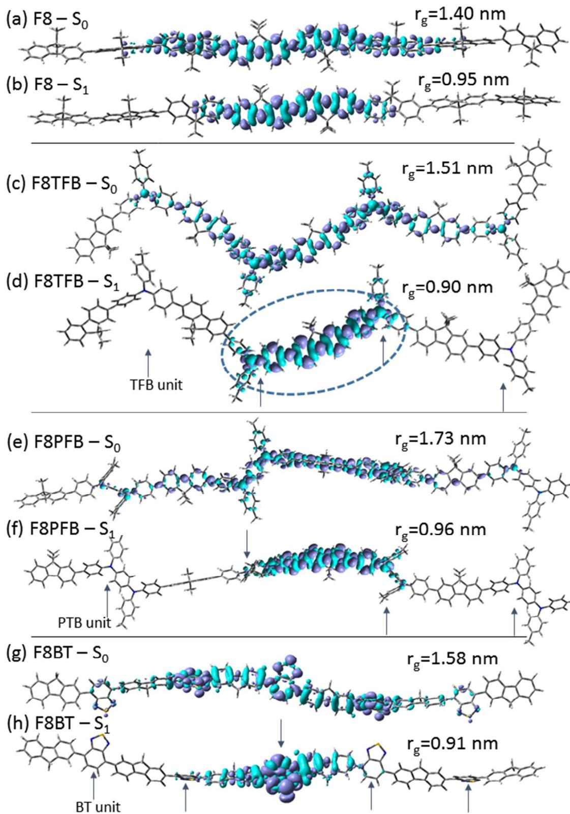
Figure 3: Plot of the electron density changes (a) (c) (e) (g) between the  $n_0$  and  $n_1$  electronic states, on the  $S_0$  geometry (absorption) and (b) (d) (f) (h) between the  $n_0$  and  $n_1$  electronic states, on the  $S_1$
