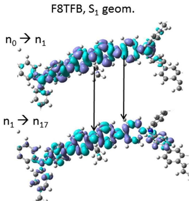
Figure 6: Zoomed in plot of the molecular portions of F8TFB circled in figures 3 and 5: the top plot is the change in electron density between the ground-state, non-excited molecule, and the first excited-state  $n_1$ ; the bottom plot is the change of electronic density between the electronic density of the first excited-state  $n_1$  and the excited-state  $n_{17}$ , corresponding to the main electronic ESA peak.
