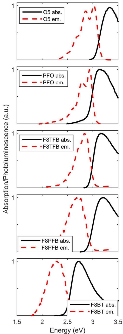
Figure 2: Experimental ground-state absorption (black solid lines) and photoluminescence (red dotted lines) spectra of fluorene pentamer, polyfluorene, F8TFB copolymer, F8PFB copolymer and F8BT copolymer in dilute solutions in toluene. Photoluminescence spectra were measured with excitation at 3.4 eV.
