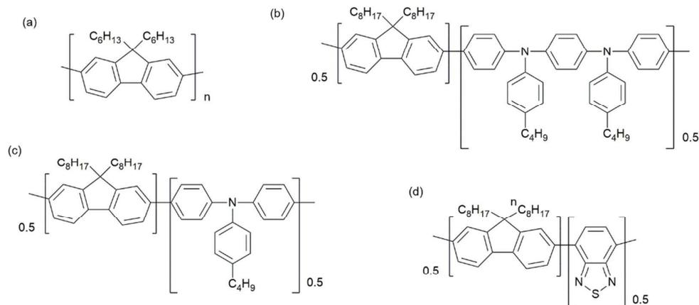
Figure 1: Sketch of the monomer units of the polymers investigated experimentally: (a) Polyfluorene (PFO), (b) F8PFB, (c) F8TFB and (d) F8BT. We have also investigated the fluorene pentamer (O5), which consists in a chain of 5 fluorene units (a), terminated by hydrogen atoms.
