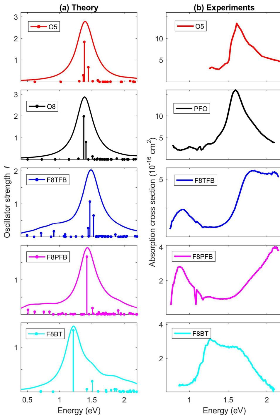
Figure 4: (a) Calculated ESA spectra for the five molecules we studied. The results presented here correspond to ESA from the first-state, in the fully-relaxed  $S_1$  molecular geometry. We used a homogeneous broadening of 150 meV. (b) Experimental ESA spectra, recorded 1ps after excitation at 3.1 eV for the five molecules we studied.
