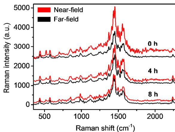
**Fig. 2** Time-series near-field and far-field spectra of a representative TERS tip measured at intervals of 4 h under ambient laboratory conditions. The plasmonic enhancement rapidly decreases after 4 h and completely disappears after 8 h of exposure to the ambient environment. Laser power at the sample: 100  $\mu$ W. Integration time: 60 s.
