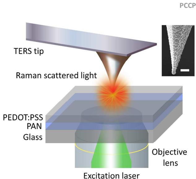
**Fig. 1** Schematic diagram of the transmission mode TERS apparatus used in this work. Tip-in (near-field) and tip-out (far-field) measurements were conducted on a bilayer sample (Top layer – poly (3, 4 ethylenedioxythiophene):poly (styrenesulfonate) (PEDOT:PSS); Bottom layer – polyacrylonitrile (PAN)) developed by Kumar *et al.*<sup>25</sup>. A scanning electron microscopy (SEM) image of a representative TERS tip is shown in the inset. Scale bar: 100 nm.
