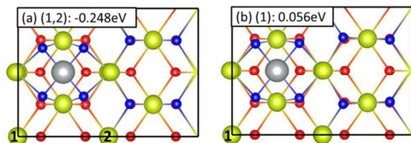
Figure 2: Adsorption of Ni on a hollow site on the CeO<sub>2</sub> (110) surface. (a) Ni is in its Ni<sup>2+</sup> oxidation state with the two Ce<sup>3+</sup> ions located at sites 1 and 2. (b) Ni is in its Ni<sup>+</sup> oxidation state with the reduced Ce<sup>3+</sup> ion located at site 1. Ce atoms are yellow, O atoms are red and blue, and Ni atom is grey.
