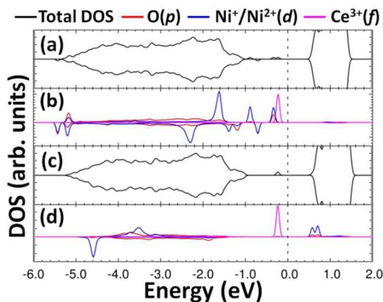
Figure 5: Total and projected density of States for the adsorption of Ni on CeO<sub>2</sub>(110) bridge site at 0.083ML coverage. (a-b) Total and projected density of states for Ni adsorbate in Ni<sup>+</sup> oxidation state. (c-d) Total and projected density of states for Ni adsorbate in Ni<sup>2+</sup> oxidation state. The Fermi level is set to 0 in all the plots.
