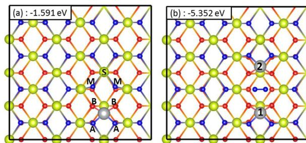
Figure 7: Ni substituent on CeO<sub>2</sub> (110) surface. (a) Optimum configuration for a mono substituent with four-coordinated Ni. (b) Optimum configuration for di Ni substituted surface. Ce atoms are yellow, O atoms are red and blue, Ni substituent is gray. 'S', 'M', 'A' and 'B' in (a) correspond to a surface Ce<sup>4+</sup> ion, magnetic oxygen atoms, surface and sub-surface oxygen atoms respectively. 1, 2 in (b) correspond to the two Ni dopants.
