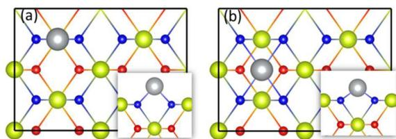
Figure 1: Initial structures of Ni adsorption on the ceria (110) surface. (a) Bridge site (b) Hollow site. Insets show the front view of the structures. Ce atoms are yellow, O atoms are red and blue, Ni atom is grey. In order to distinguish the surface O atoms from other O atoms in the slab, they are shown in blue colour.
