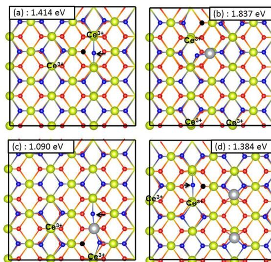
Figure 9: Active oxygen vacancy on (a) pure, (b) Ni adsorbed, (c) Mono-Ni substituted and (d) di-Ni substituted  $\text{CeO}_2$  (110) surface.  $\text{Ce}^{4+}$  ions are yellow,  $\text{Ce}^{3+}$  ions are blue,  $\text{O}^{2-}$  ions are red and  $\text{Ni}^+/\text{Ni}^{2+}$  ions are grey. The position of the oxygen vacancy is shown by black spheres. Arrows in (a), (c) and (d) show the motion of an oxygen atom from its surface site to a bridging position.
