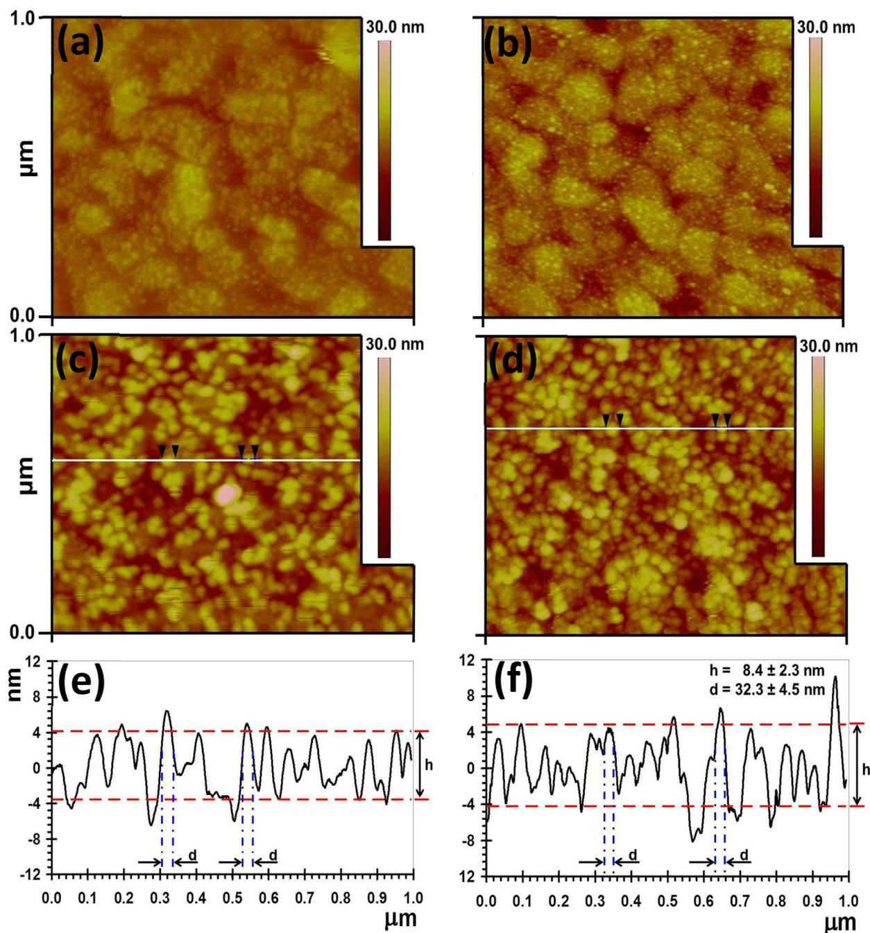
**Figure 2.** AFM images showing the surface topographies of: a) C11-thiol SAM/Au and b) C9-thiol SAM/Au substrates (background) as well as those for the respective: c) PS I/C11-thiol SAM/Au and d) PS I/C9-thiol SAM/Au substrates. Representative cross-sectional surface profiles (e & f) for PS I assembled SAM/Au substrates are shown below the respective AFM images (c & d).
