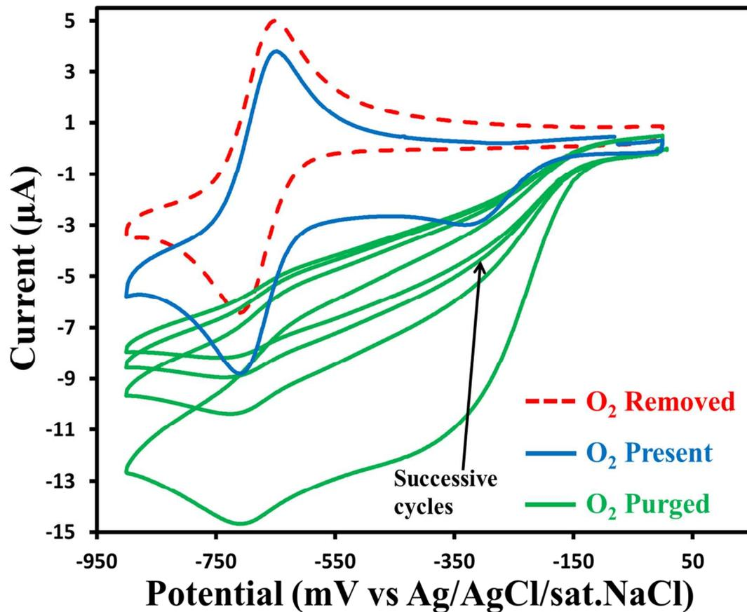
**Figure 7.** Cyclic Voltammetry scans at 200 mV/s on PS I/C9-thiol SAM/Au electrodes vs Ag/AgCl in dark with 1 mM MV in solution. When purged with nitrogen to remove all oxygen, the scans exhibited a stable repeated single redox peak for MV at the expected potential of  $\sim -0.65$  V. When pure oxygen is bubbled through the solution, the irreversible redox peak appears grows in magnitude, while the distinguishable  $MV^+/MV^{2+}$  pair diminishes by  $\sim 50\%$  peak to peak height.
