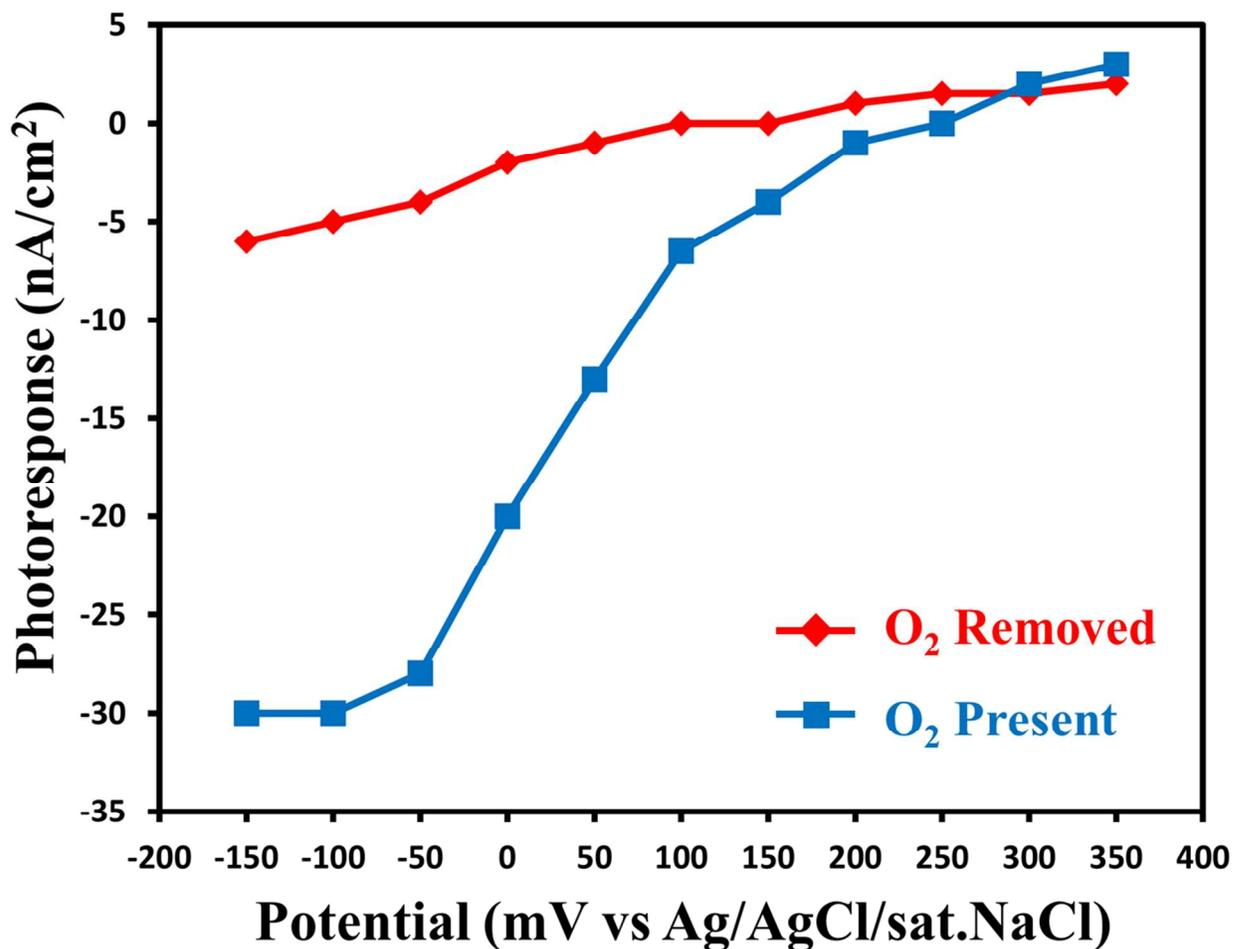
**Figure 8.** Net photocurrent change in series of continuous chronoamperometry biased steps on dropcast PS I/GC electrodes under illumination ( $\lambda = 635 - 650$  nm) with 1 mM methyl viologen (MV) added as charge carrier under aerobic and anaerobic conditions.
