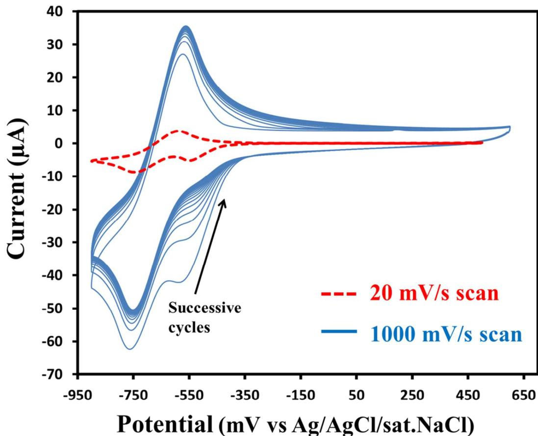
**Figure 6.** Cyclic Voltammetry scans on PS I/C9-thiol SAM/Au electrodes vs Ag/AgCl in dark with 1 mM MV in solution in aerobic conditions. Immediately stable trace at 20 mV/s scan and greatly diminishing reduction peak at 1000 mV/s scan indicates a methyl viologen-oxygen complex being formed in solution and consumed at the electrode surface.
