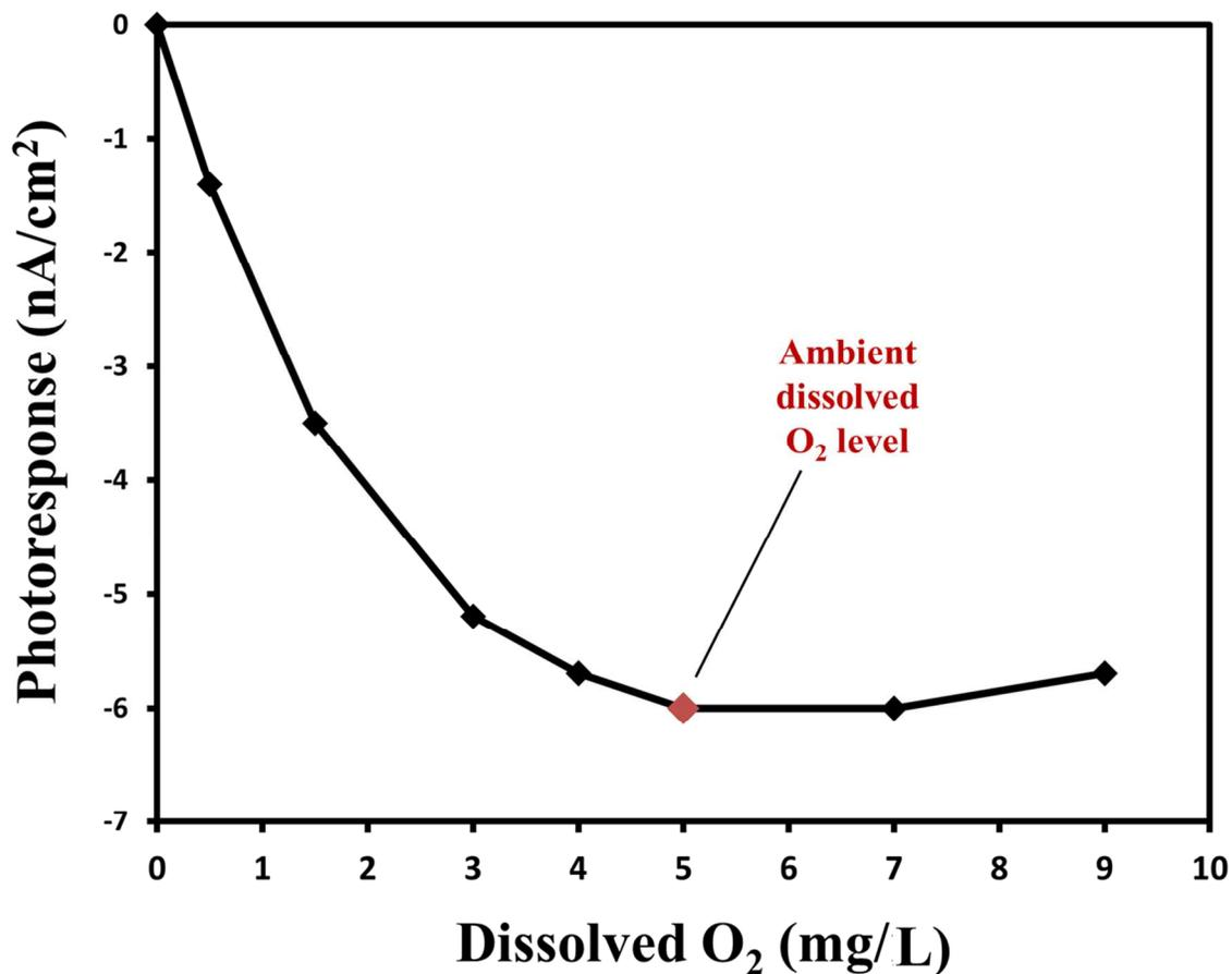
**Figure 4.** Net photocurrent change in series of chronoamperometry on PS I/C9-thiol SAM/Au electrodes at +0 V bias vs Ag/AgCl under illumination ( $\lambda = 635 - 650$  nm) with 1 mM methyl viologen. O<sub>2</sub> concentration heavily regulates the scavenging of electrons from PS I. For the given concentration of MV, adding oxygen beyond the ambient amount present in Millipore deionized water did not further increase the photoresponse of PS I.
