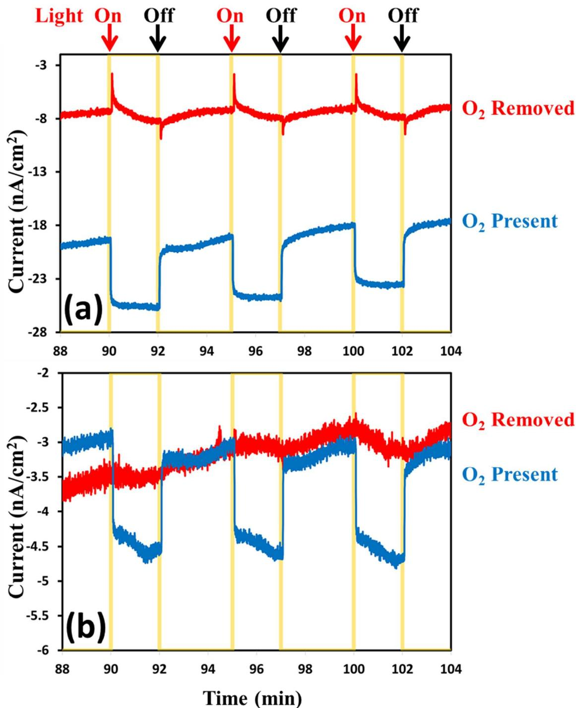
**Figure 3.** Chronoamperometry on PS I/C9-thiol SAM/Au electrodes at +0 V bias vs Ag/AgCl under illumination ( $\lambda = 635 - 650$  nm) under both aerobic (O<sub>2</sub> present; blue line) and anaerobic (O<sub>2</sub> absent; black line) conditions with: a) 1 mM methyl viologen (MV) added as charge carrier showing suppression of photocurrent with O<sub>2</sub> removed; b) all charge carrier removed from solution, showing small direct scavenging of electrons by O<sub>2</sub>.
