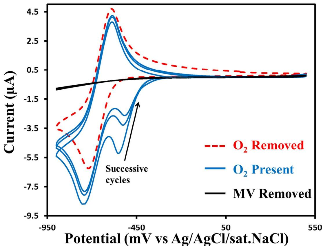
**Figure 5.** Cyclic Voltammetry scans at 200 mV/s on PS I/C9-thiol SAM/Au electrodes vs Ag/AgCl in dark with 1 mM MV in solution. When purged with nitrogen to remove all oxygen, the scans exhibited a stable repeated single redox peak for MV at the expected potential of  $\sim -0.65$  V. When oxygen is introduced, an irreversible redox peak appears that diminishes in magnitude upon successive scans, which is attributed to the reduction of the metastable methyl viologen-oxygen complex.
