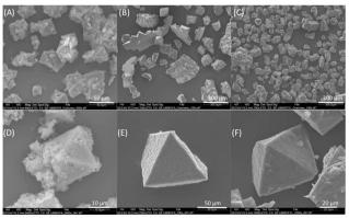
Figure 2. SEM images of bulk phases of (A) UBMOF-8, (B) UBMOF-9, (C) UBMOF-31 and their close up views D, E, and F, respectively.
