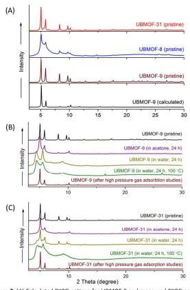
Figure 3. (A) Calculated PXRD pattern for UBMOF-9 and measured PXRD patterns for pristine UBMOF-8, UBMOF-9, and UBMOF-31 suggesting the phase-pure bulk material for UBMOF 9 and UBMOF-31. (B, C) Comparison of PXRD patterns of UBMOF-9, and UBMOF-31 treated at different conditions.
