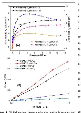
Figure 4. (A) High-pressure hydrogen adsorption studies (gravimetric and volumetric) for UBMOF-9 and UBMOF-31. (B) Study of CO<sub>2</sub> adsorption and N<sub>2</sub> adsorption showing greater affinity of UBMOF-31 for CO<sub>2</sub> over N<sub>2</sub>, compared to UBMOF-9 at 1 MPa and 0 °C.
