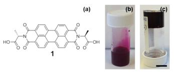
Figure 1. (a) Structure of PBI 1; (b) Photograph of a solution of 1 in water at pH 9 at 5 mg/mL; (c) Photograph of the corresponding gel at pH 4.
