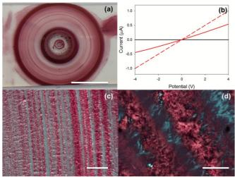
Figure 3. (a) Photograph of dried solution of 1 after shearing for 16 hours. Scale bar represents 1 cm. (b) Photoresponse of the shear aligned dried solution of 1. Black data is in the dark and red data is under 365 nm light. Solid red data is against alignment and red datab data is with alignment. (c) and (d) Optical microscope images of (a) viewed under cross-polarised light. The scale bars in (c) and (d) correspond to 0.2 mm and 50 µm, respectively.
