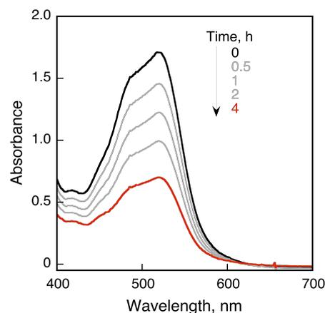
**Fig. 1** Visible absorption change in photocatalytic oxidation of [Fe<sup>II</sup>(bpy)<sub>3</sub>]<sup>2+</sup>(PF<sub>6</sub><sup>-</sup>)<sub>2</sub> (2.0 mM) by O<sub>2</sub> in O<sub>2</sub>-saturated MeCN in the presence of [Acr<sup>+</sup>-Mes](ClO<sub>4</sub><sup>-</sup>) (0.20 mM) and HOTf (0.10 M) at 298 K under visible light irradiation with a xenon lamp with a cut filter (λ > 390 nm).
