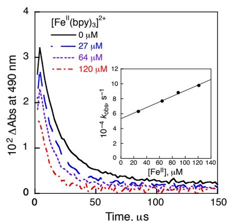
**Fig. 3** Transient absorption decay at 490 nm due to the electron-transfer state of [Acr<sup>+</sup>-Mes](ClO<sub>4</sub><sup>-</sup>) with various concentrations of [Fe<sup>II</sup>(bpy)<sub>3</sub>]<sup>2+</sup>(PF<sub>6</sub><sup>-</sup>)<sub>2</sub>. Inset: decay rate constant versus concentrations of [Fe<sup>II</sup>(bpy)<sub>3</sub>]<sup>2+</sup>(PF<sub>6</sub><sup>-</sup>)<sub>2</sub>.
