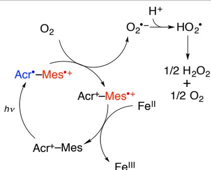
**Scheme 1** Photocatalytic cycle for oxidation of iron(II) complexes to iron(III) complexes by O<sub>2</sub> with Acr<sup>+</sup>-Mes.
