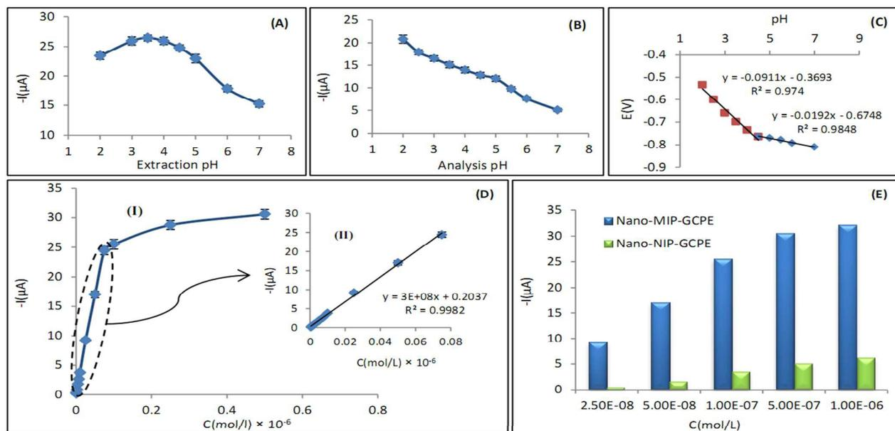
**Fig. 3** Effect of Extraction pH(A), and Analysis pH(B & C), on the SWV response of modified CPE after extraction from  $5.0 \times 10^{-7}$  M CDP solution. (D) The calibration curve (I) and linear range related to it (II), obtained for developed method. (E) Comparison of SWV responses obtained at nano-MIP and nano-NIP based sensors under optimum conditions.
