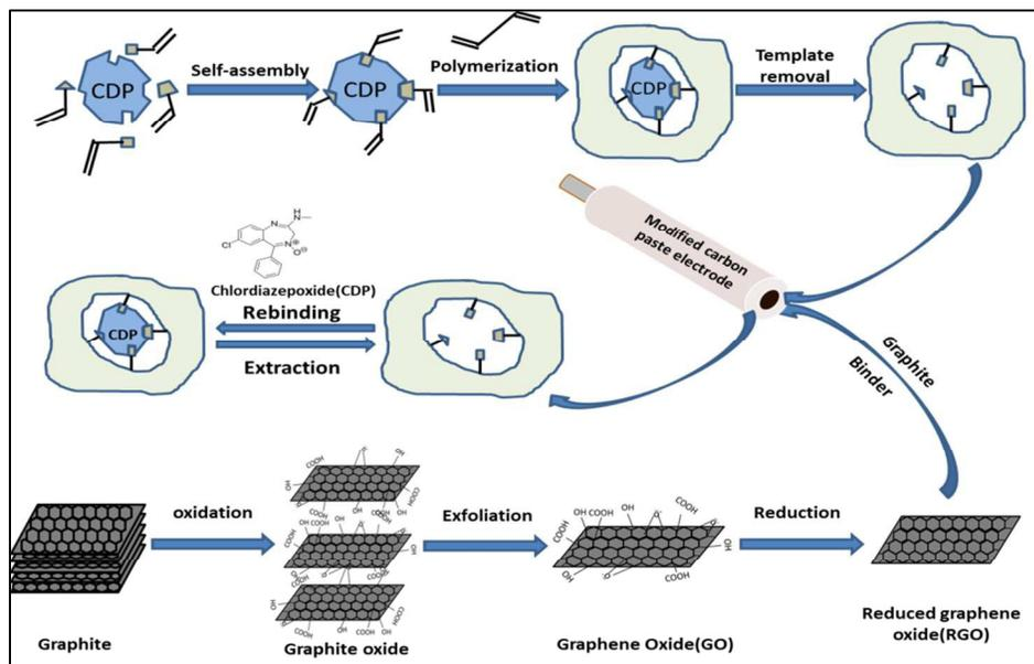
In this study, we introduce a Molecularly imprinted polymer for chlordiazepoxide(CDP) drug with improved properties through the preparation of MIP particles at nano-dimension and its use for modification of Graphene-carbon paste electrode to preparation of new electrochemical sensors for selective and sensitive determination of CDP.
