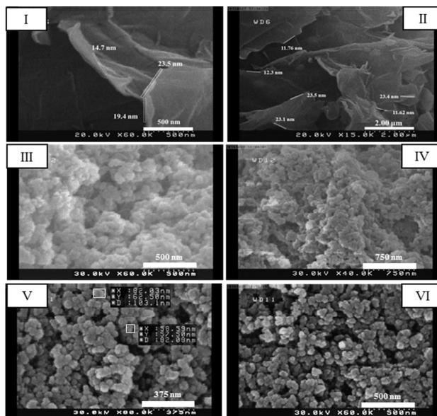
Fig. 1 Scanning electron microscopy images of graphene nanosheets (I & II), microparticles (III & IV) and nanoparticles (V – VI) of MIP.
