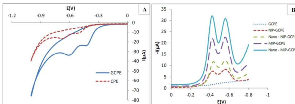
**Fig. 2** (A) Cyclic voltammetry behaviour of  $5.0 \times 10^{-5}$  M CDP solution on the CPE and GCPE. (B) Square wave voltammetric signals of GCP and modified GCP electrodes after 10 min extraction from  $1.0 \times 10^{-6}$  M CDP solutions (pH= 4.5). (The SW conditions:  $\Delta E= 20$  mV,  $V_{step}= 5$  mV,  $t_{step} = 0.3$  s, Frequency = 20 Hz)
