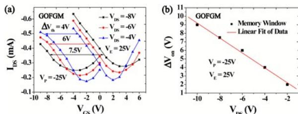
Fig. 3 (a) Memory hysteresis behavior of the GOFGM as a function of the  $V_{DS}$  at  $-4$  V,  $-6$  V,  $-8$  V; (b) Memory window of the GOFGM as a function of the  $V_{DS}$  bias.
