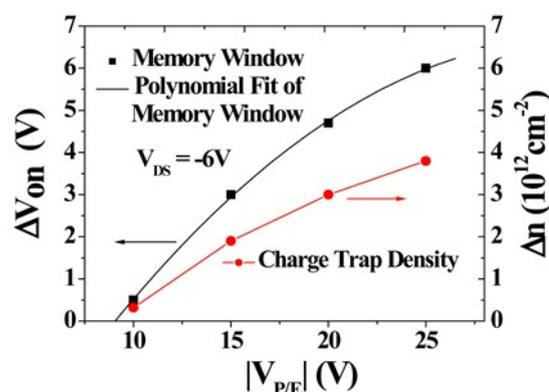
Fig. 4 Memory window (black dots), polynomial fit of memory window (black line) and charge trap density (red dots) versus the  $V_{P/E}$  sweep range.
