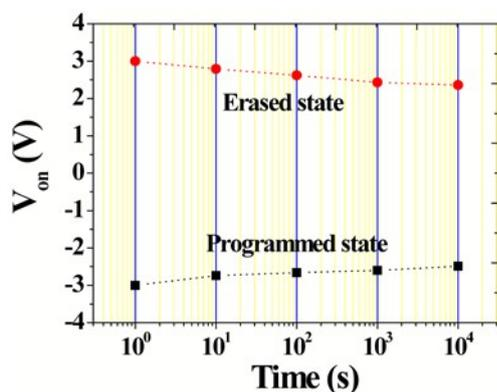
Fig. 5 Programming (black dots)/erasing (red dots) data retention properties as a function of the retention time.
