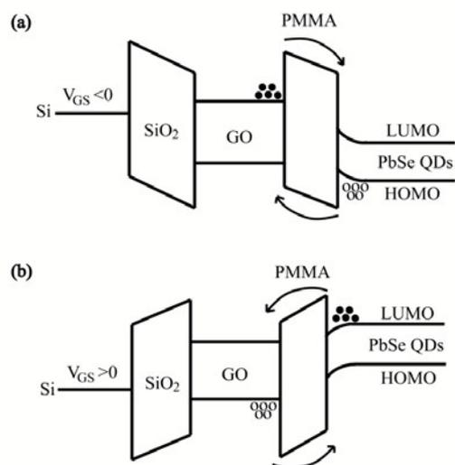
Fig. 6 Energy level diagrams with supplying negative  $V_{GS}$  (a) and positive  $V_{GS}$  (b).
