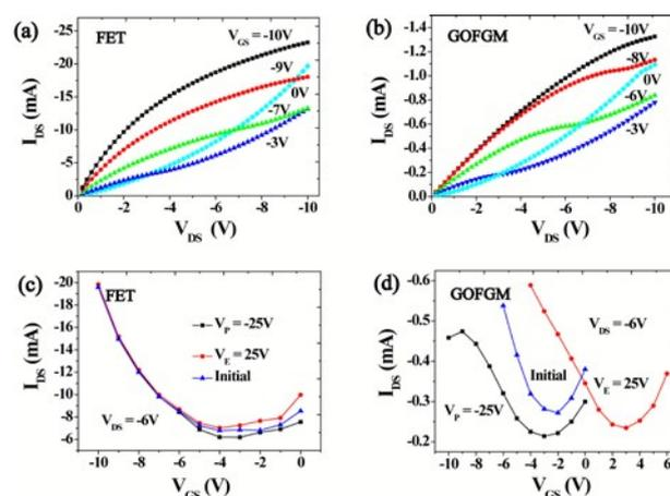
Fig. 2 Output characteristics of the FET (a) and the GOFGM (b) at the initial state. Transfer characteristics of the FET (c) and the GOFGM (d) after  $V_p/\epsilon$  at  $-/+25$  V at  $V_{DS}$  of  $-6$  V.
