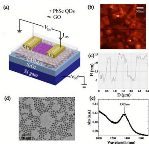
Fig. 1 (a) Schematic diagram of the ambipolar GOFGM; (b) AFM of GO deposited on  $n^+$  Si/SiO<sub>2</sub> substrate; (c) The height of GO film; (d) TEM of PbSe QDs; (e) Light absorbance of PbSe QDs.
