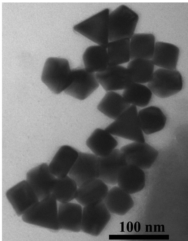
Fig. 4c: The TEM image of the separated supernatant upon the addition of CTAC in the secondary process.
