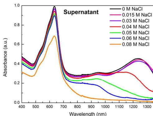
Fig. 6b: The absorption spectra of separated supernatant after the addition of different concentration of NaCl, the concentration of NaCl is ranging from 0.015 M to 0.08 M.
