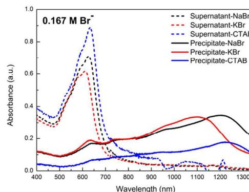
Fig. 7a: The absorption spectra of supernatant and precipitate separated by NaBr, KBr and CTAB. (0.167 M Br<sup>-</sup>)
