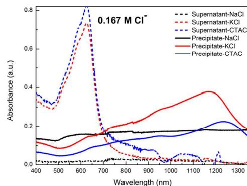
Fig. 6a: The absorption spectra of supernatant and precipitate separated by NaCl, KCl and CTAC. (0.167 M  $\text{Cl}^-$ )
