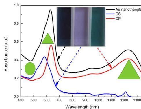
Fig. 3d: The absorption spectra of as-prepared gold nanotriangles before and after the addition of CTAC, the inset: the corresponding color. (CS denotes supernatant, CP denotes
