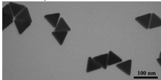
Fig. 5c: The TEM image of the separated supernatant upon the addition of CTAB in the secondary process.
