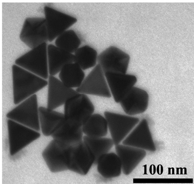
Fig. 3b: The TEM image of the separated supernatant upon the addition of CTAB.
