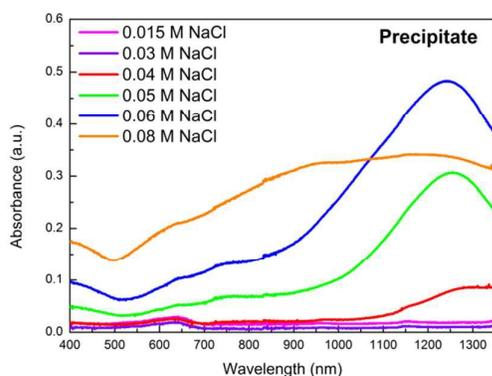
Fig. 6c: The absorption spectra of separated precipitate after the addition of different concentration of NaCl, the concentration of NaCl is ranging from 0.015 M to 0.08 M.
