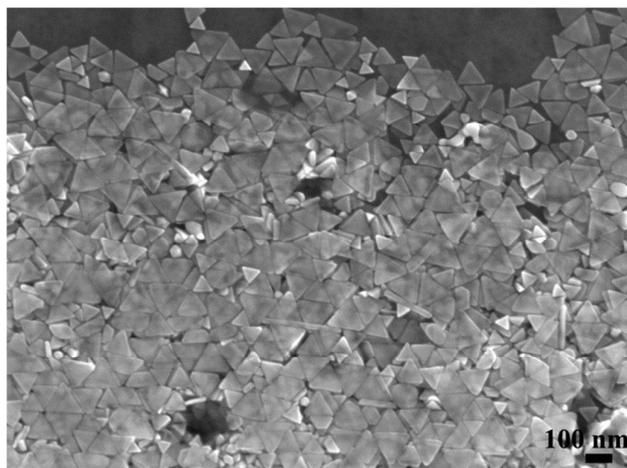
Fig. 5f: The SEM image of the separated gold nanotriangles with a large size.
