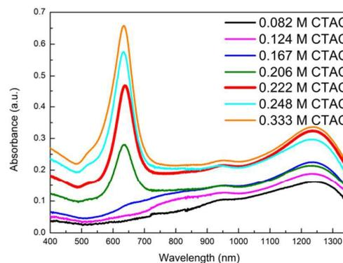
Fig. 2d: The absorption spectra of the precipitate of gold nanotriangles after the addition of different concentration of CTAC.
