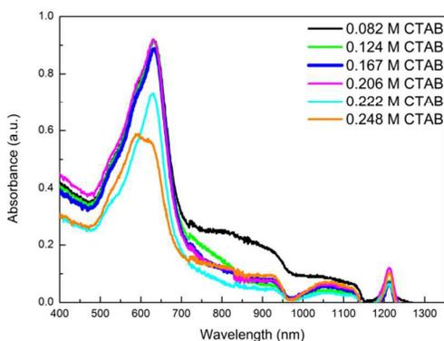
Fig. 2a: The absorption spectra of the supernatant of gold nanotriangles after the addition of different concentration of CTAB.
