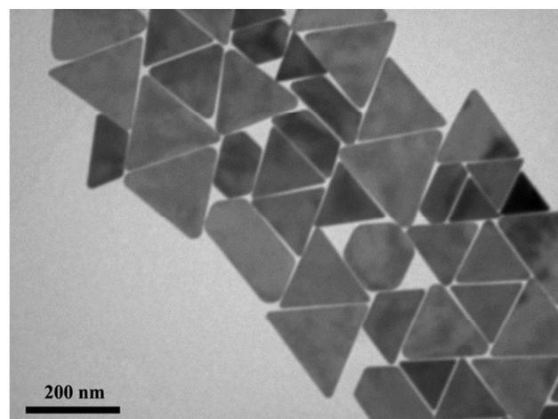
Fig. 3f: The TEM image of the separated precipitate upon the addition of CTAC.
