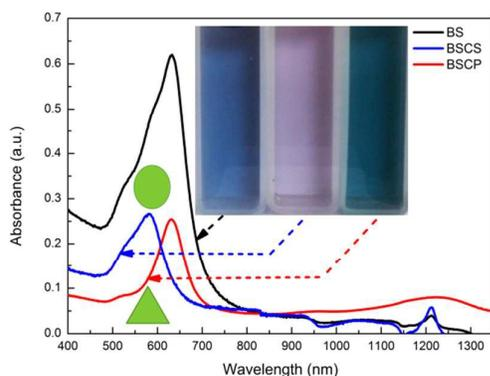
Fig. 4b: The absorption spectra of CTAB-separated supernatant before and after the addition of CTAC, the inset: the corresponding color. (BS denotes the CTAB-separated supernatant, BSCS denotes the supernatant of BS after the addition of CTAC, BSCP denotes the precipitate of BS after the addition of CTAC).
