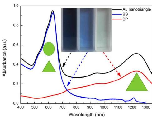
Fig. 3a: The absorption spectra of as-prepared gold nanotriangles before and after the addition of CTAB, the inset: the corresponding color. (BS denotes supernatant, BP denotes precipitate).
