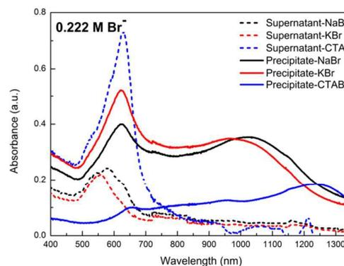
Fig. 7b: The absorption spectra of supernatant and precipitate separated by NaBr, KBr and CTAB. (0.222 M Br<sup>-</sup>)
