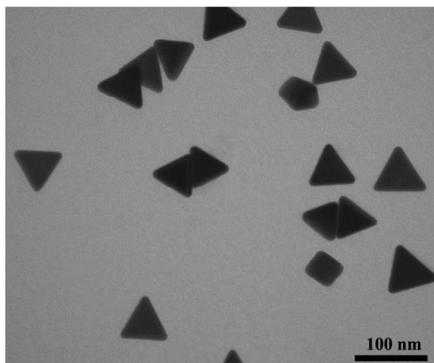
Fig. 4d: The TEM image of the separated precipitate upon the addition of CTAC in the secondary process.
