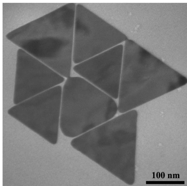
Fig. 5d: The TEM image of the separated precipitate upon the addition of CTAB in the secondary process.
