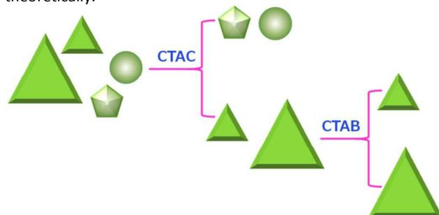
Fig. 5a: A schematic illustration of separation nanotriangles with high purification based on CTAB and CTAC through a two-step strategy. (Approach 2)
