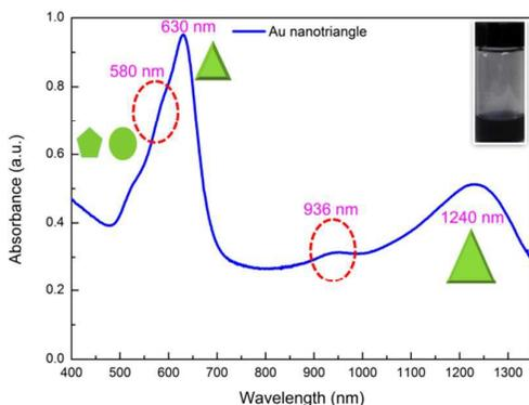
Fig. 1a: The absorption spectrum of the as-prepared gold nanotriangles.
