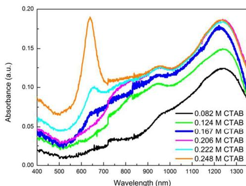
Fig. 2b: The absorption spectra of the precipitate of gold nanotriangles after the addition of different concentration of CTAB.
