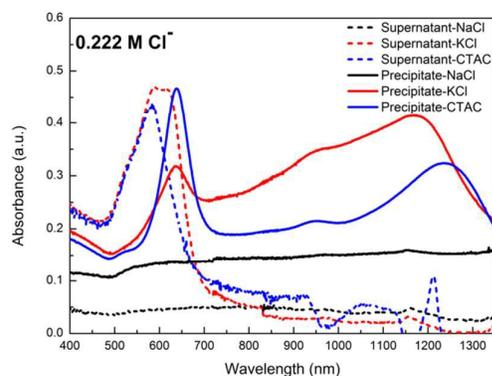
Fig. 6d: The absorption spectra of supernatant and precipitate separated by NaCl, KCl and CTAC. (0.222 M Cl<sup>-</sup>).
