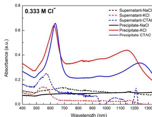
Fig. 6e: The absorption spectra of supernatant and precipitate separated by NaCl, KCl and CTAC. (0.333 M Cl<sup>-</sup>).
