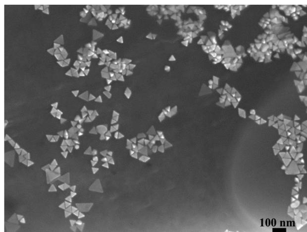
Fig. 5e: The SEM image of the separated gold nanotriangles with a small size.
