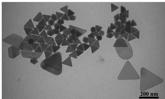
Fig. 1b: The typical TEM image of the as-prepared gold nanotriangles.
