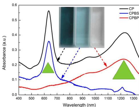
Fig. 5b: The absorption spectra of CTAC-separated precipitate before and after the addition of CTAB, the inset: the corresponding color. (CP denotes the CTAC-separated precipitate, CPBS denotes the supernatant of CP after the
