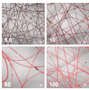
**Fig. 4** Confocal images of fibres obtained from PMMA<sub>solut</sub>-Mo<sup>x</sup>, where x = 5.0, 10, 50 or 100. The white scale bars represent 30  $\mu$ m.
