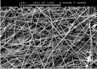
Fig. 3 SEM image of the electrospun fibres of PMMA<sub>solut</sub>-Mo<sup>100</sup>
