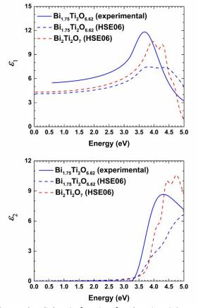
**Fig. 5.** The dielectric function for the  $Bi_{1.75}Ti_2O_{6.62}$  structure measured via spectroscopic ellipsometry (solid blue line) and those calculated using the HSEO6 functional for the same non-stoichiometric structure (dashed blue) and for the stoichiometric  $Bi_2Ti_2O_7$  compound (red line).
