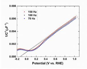
FIG. 7. Mott-Schottky plot for non-stoichiometric Bi<sub>1.75</sub>Ti<sub>2</sub>O<sub>6.62</sub>.
