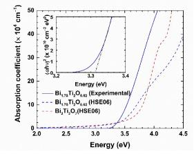
**Fig. 6.** Absorption coefficients of the spectra of  $Bi_{1.75}Ti_2O_{6.62}$  obtained via ellipsometric spectroscopy (solid blue) and computed using the HSEO6 functional, together with the results computed for  $Bi_2Ti_2O_7$ . The inset shows the Tauc plot of the measured results for  $Bi_{1.75}Ti_2O_{6.62}$ .
