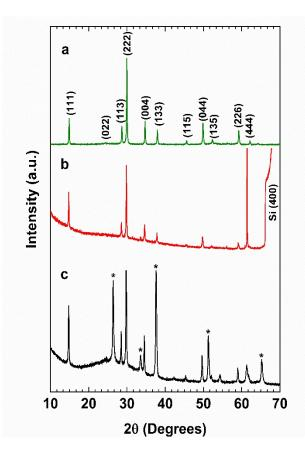
Fig. 2. XRD patterns of a)  $Bi_{1.75}Ti_2O_{6.62}$  powders, b) a  $Bi_{1.75}Ti_2O_{6.62}$  thin film on a Si substrate, and c) a  $Bi_{1.75}Ti_2O_{6.62}$  thin film on an FTO substrate.
