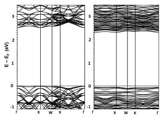
**Fig. 4.** Electronic band structure diagrams along the highsymmetry *k*-points obtained using the PBE functional for (a) stoichiometric  $Bi_2Ti_2O_7$  and (b) non-stoichiometric  $Bi_{1.75}Ti_2O_{6.62}$ ,  $E_F$  is set at 0 eV.
