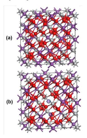
**Fig. 1.** DFT-optimized lowest-energy structures obtained using the PBE functional for (a) perfect  $Bi_2Ti_2O_7$  and (b) defectcontaining  $Bi_{1.75}Ti_2O_{6.62}$  material with aggregated Bi and O vacancies. Color legend: Bi in purple, Ti in gray, O in red, and Bi (O) vacancies in dotted circles.
