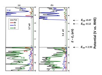
**Fig. 3**. Electronic DOSs obtained using the HSE06 functional for (a) stoichiometric  $Bi_2Ti_2O_7$  and (b) non-stoichiometric  $Bi_{1.75}Ti_2O_{6.62}$  material in their most stable configurations, as reported in Fig. 2. Color legend: total DOS in black; DOSs projected onto Bi in red, onto Ti in blue, and onto O atoms in green. Potentials for valence band edge, conduction band edge, and flatband estimated from Mott-Schottky analysis are also represented in RHE scale (pH 13.2).
