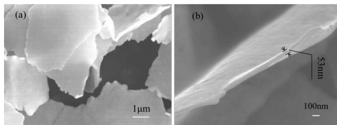
**Fig.3** SEM images of silver flakes ultrasonically treated for 60min (a) surface topography; (b) cross-section.
