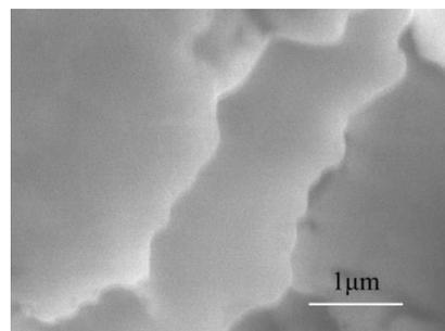
Fig.7 SEM image of ECAs patterns (filled with 25 wt% of as-prepared silver flakes) printed on PET substrate.
