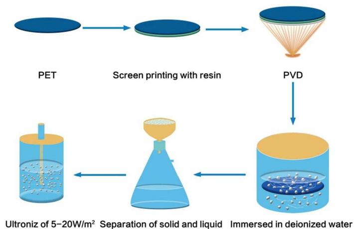
Flaky silver powders with nano-thickness and smooth surface were prepared through nanofilm transition method which production process is environmental-friendly.
