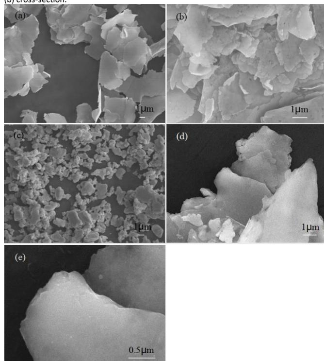
**Fig.4** SEM images of silver powders (a) As-prepared (b) Xinshengfeng (c) FAGL 6501 (d) Acheson ED 427SS (e) sideward thickness of Acheson ED 427SS.
