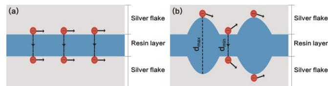
Fig.8 Conductive model of different flaky silver powders (a) as-prepared; (b) commercially available.
