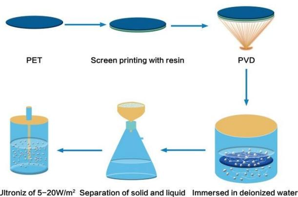
**Fig.1** Fabrication of flaky silver powders through nanofilm transition method.
