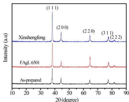
Fig.5 X-ray diffraction (XRD) patterns of flaky Ag powders.
