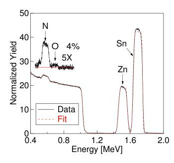
Figure 10: Oxygen impurity concentration in a nominally stoichiometric film grown at 230°C was determined by RBS to be 4%. Assuming every oxygen forms an  $O_N$  defect, this level of oxygen impurities suggests at least 2%  $V_N$  defects to satisfy the 10% Zn-rich composition for which *n*-type carrier density of 3 x 10<sup>18</sup> cm<sup>-3</sup> was observed.
