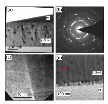
Figure 6: Bright field TEM (a) of a stoichiometric sample grown at 300°C shows columnar grain structure, consistent with SEM. A corresponding TED pattern (b) shows polycrystalline morphology and some preference for growth along [0001]. A top-down HRTEM image (c) for the same sample shows atomicscale crystallinity and grain boundaries free from precipitates. Panel (d) is an HAADF image that when paired with EDX showed evidence of nanovoids at the grain boundaries (indicated by a red arrow).
