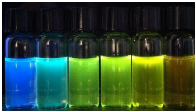
Fig. 2 Positive solvatochromism displayed by 4 upon increasing solvent polarity under UV irradiation (from left to right: n -hexanes, toluene, EtOAc, THF, DCM, acetone.)
